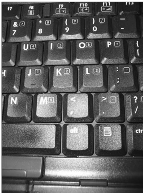
Figure 2-10: Most laptops have a built-in number pad that you activate with the Fn key.
