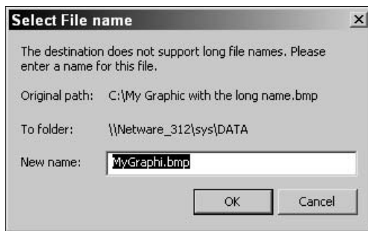
Figure 4-1: When copying files, you may be prompted to rename files if the destination does not support long filenames.
