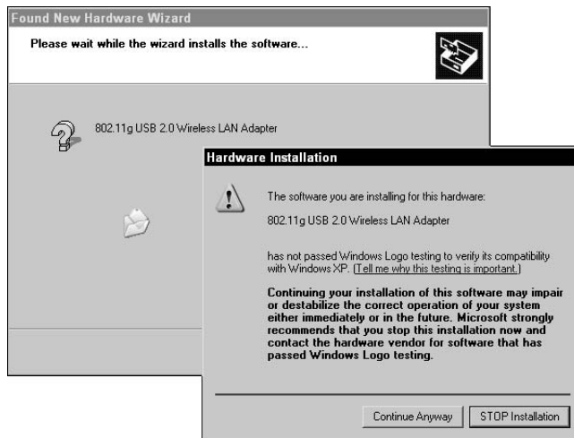
Figure 1-7: Driver Signing prevents the installation of unwanted drivers.
