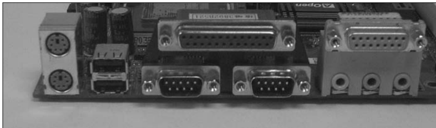
Figure 1-11: Looking at the built-in ports on the back of an ATX motherboard.
