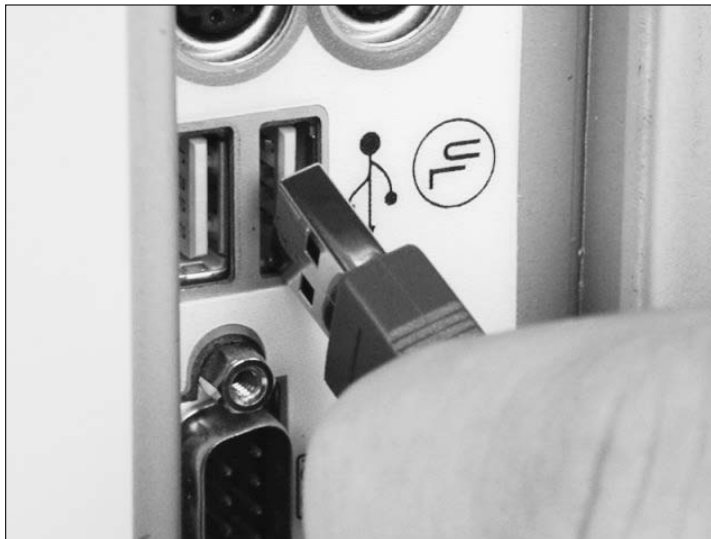
Figure 2-4: A USB keyboard connects to a USB port on the system.
