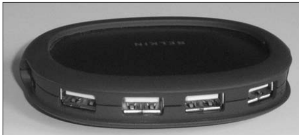
Figure 1-19: A USB hub with four ports.
