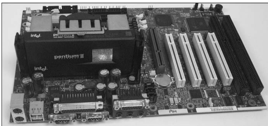
Figure 1-3: Looking at a Pentium II using the SEC packaging.
