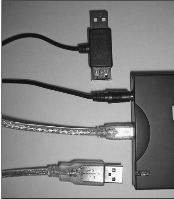
Figure 2-7: Here is a device powered by two USB ports, using a pass-through connector for the second port.
