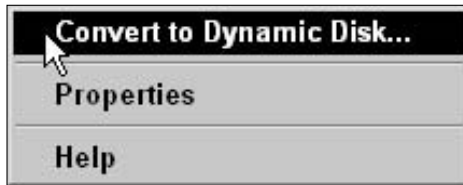
Figure 5-26: Converting a basic disk to a dynamic disk.
