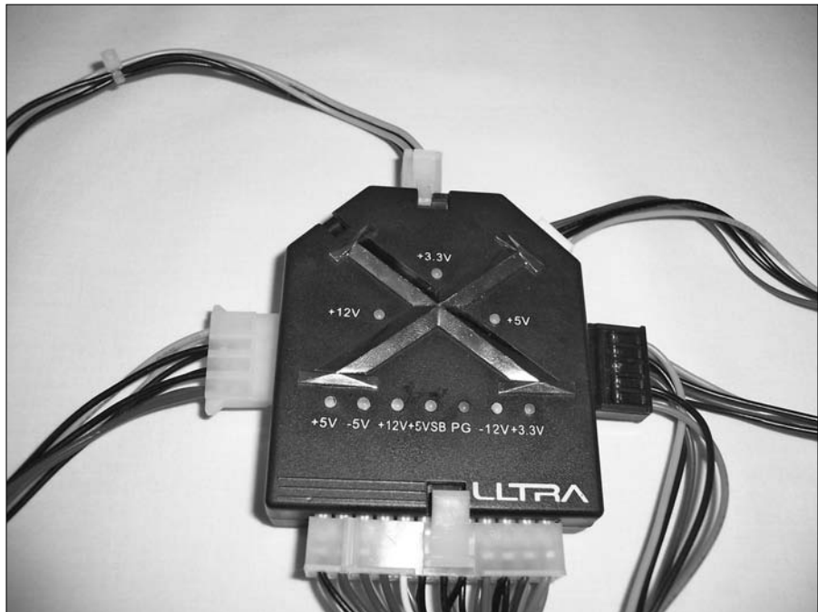
Figure 2-8: A power supply tester can save time when testing voltage supplied by power supplies.
