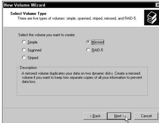
Figure 5-35: Selecting a mirrored volume type when creating a new volume.
