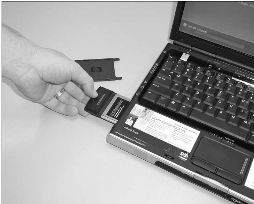
Figure 7-5: Inserting a PCMCIA card into the PCMCIA slot.
