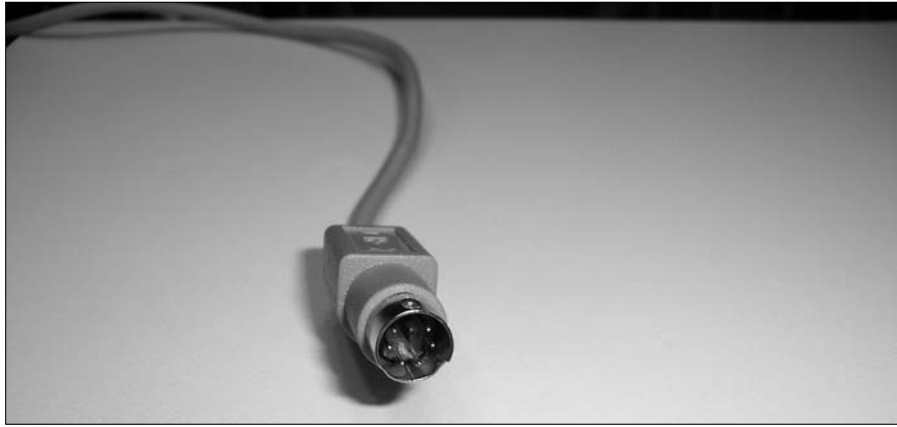
Figure 1-11: PS/2 connectors are used for keyboards and mice.
