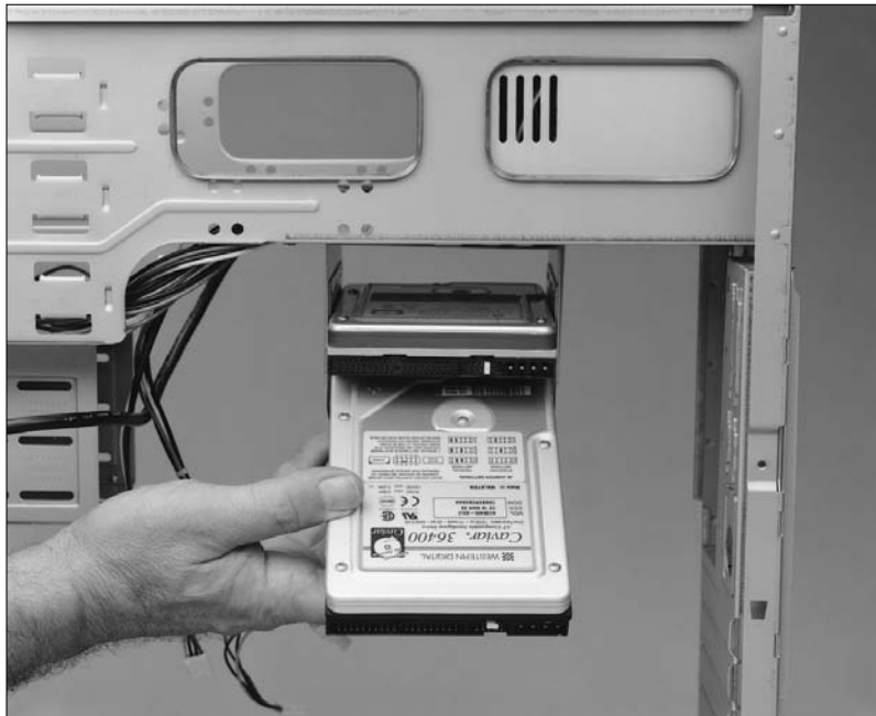
Figure 5-6: Mounting the hard disk into the drive bay.
