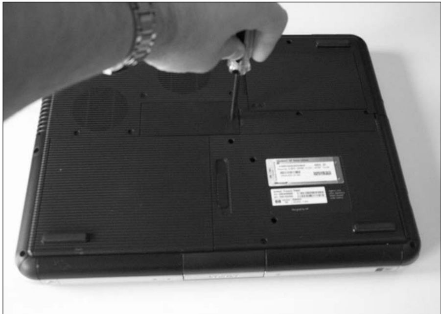
Figure 3-8: Removing the cover to add memory to a laptop.
