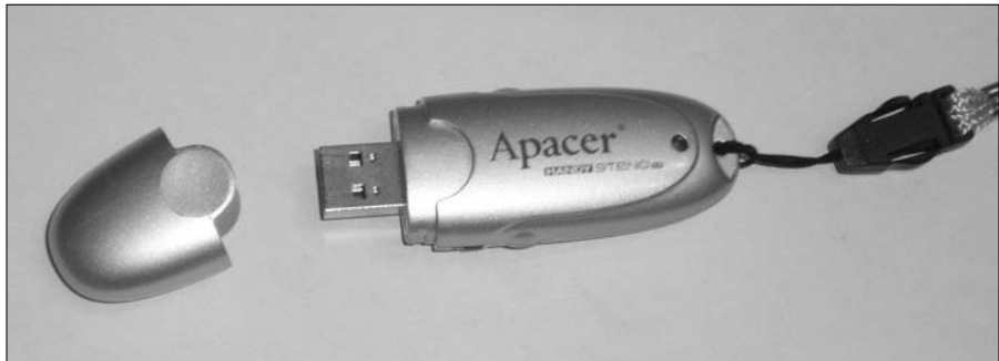
Figure 5-19: A flash drive uses a USB connection to interface with the computer.
