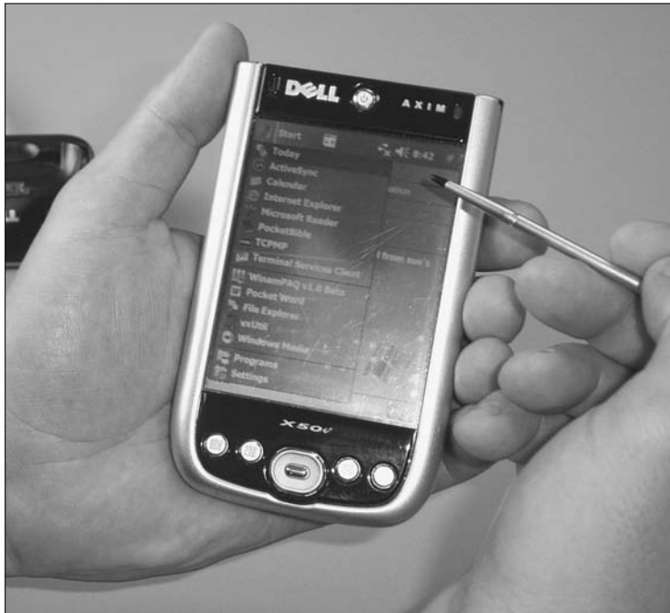
Figure 7-9: A PDA being controlled by a stylus.
