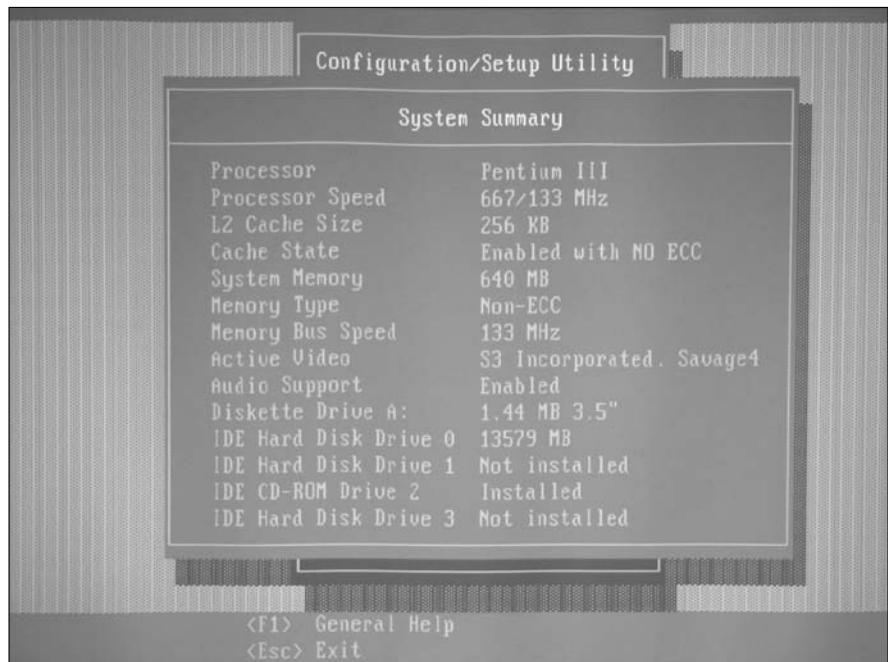
Figure 4-7: Viewing the amount of memory installed on the system through CMOS.
