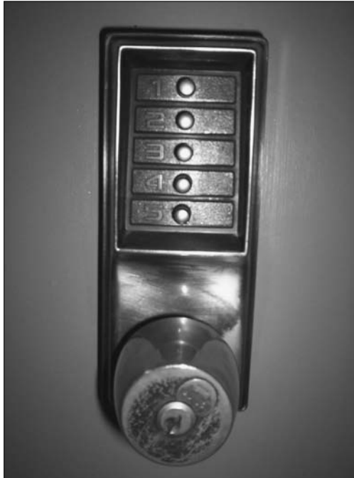
Figure 1-4: A numeric keypad used to enforce physical security.
