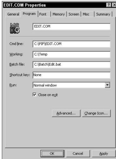
Figure 2-9: The Program tab allows you to specify information related to the executable file.
