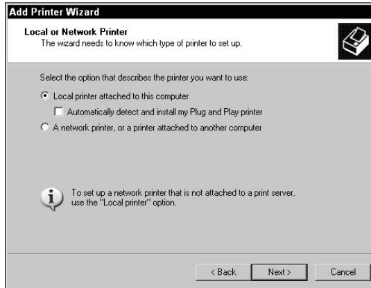
Figure 5-8: Installing a local printer in Windows XP.
