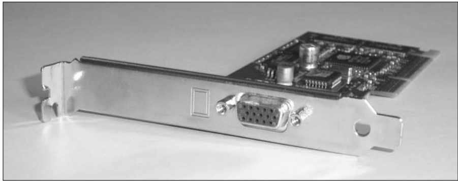
Figure 3-1: Looking at the back of a video card and the port style.
