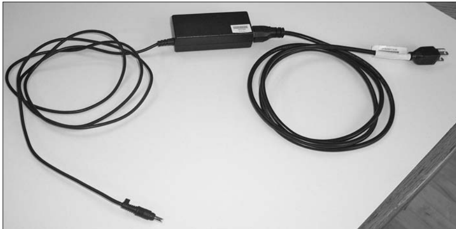
Figure 7-3: Looking at an AC adapter that supplies power to the laptop and charges the battery.
