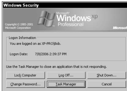
Figure 2-4: The Security dialog box for Windows XP allows you to launch Task Manager.
