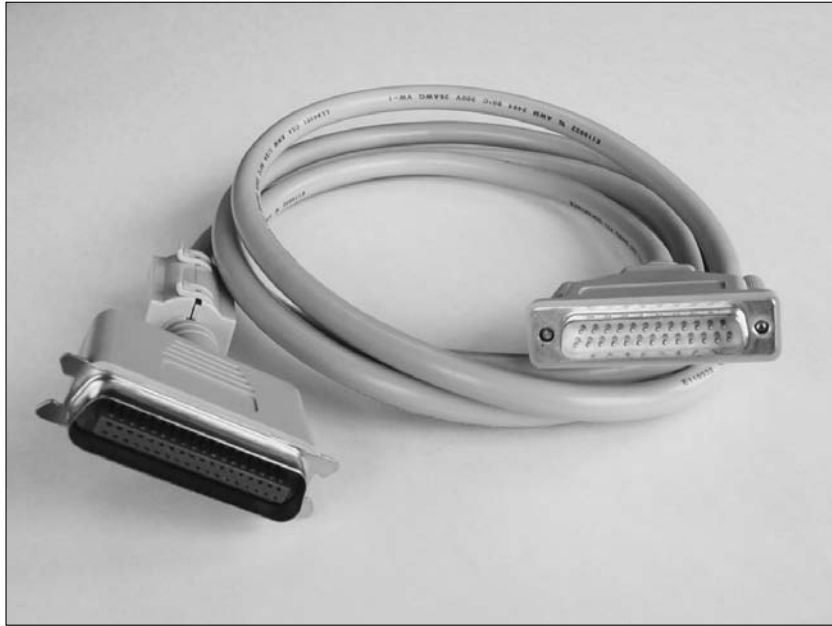
Figure 5-6: A parallel cable uses a 25-pin/36-pin connector on either end of the cable.
