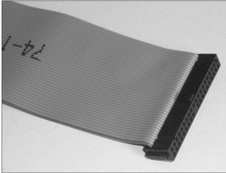
Figure 1-25: A 40-wire IDE ribbon cable.
