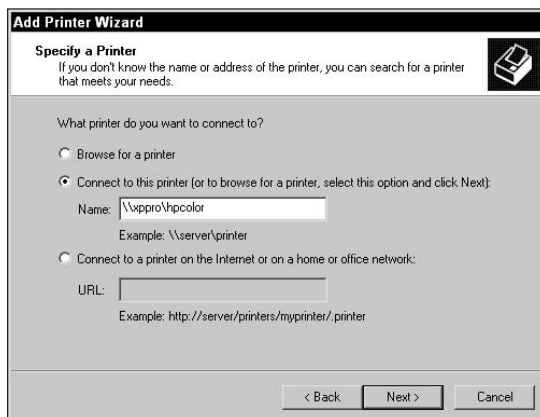
Figure 5-12: Connecting to a shared printer.
