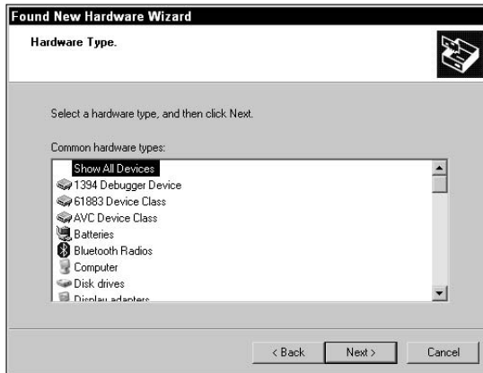
Figure 1-2: Choose the type of device you are installing so that you can look at a filtered list.
