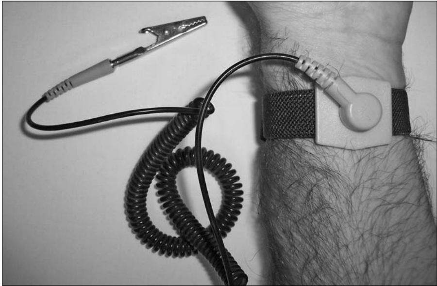
Figure 2-2: An anti-static wrist strap with a removable clip, allowing the plug to be used with some hardware.
