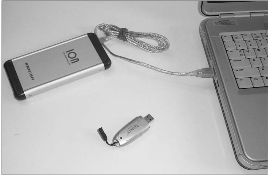
Figure 7-8: You can add storage space by using a USB external hard disk (top) or a USB flash drive (bottom).
