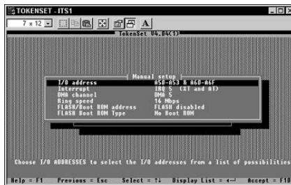
Figure 4-15: Changing resources on a non-Plug and Play device using the setup disk.
