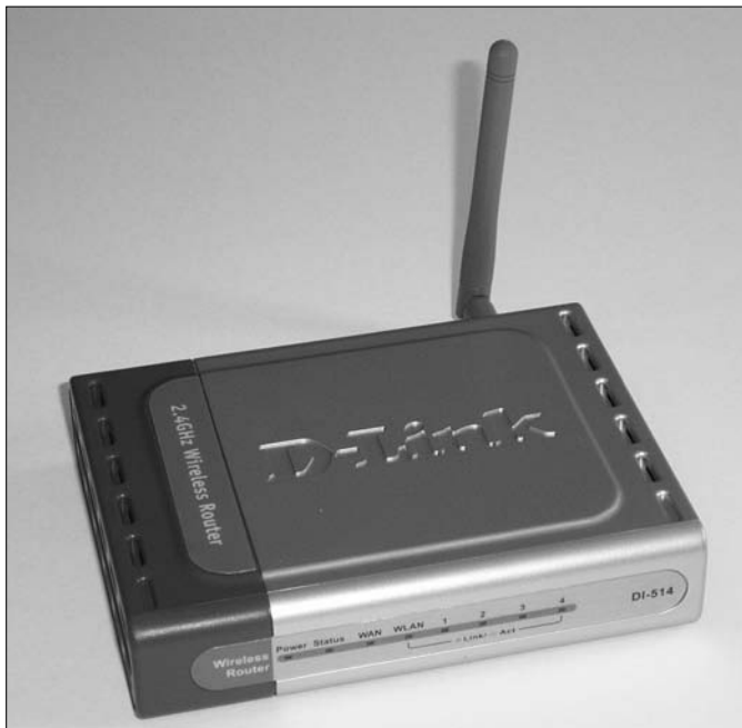
Figure 1-27: A four-port wireless router also contains a WAN link for the Internet connection.
