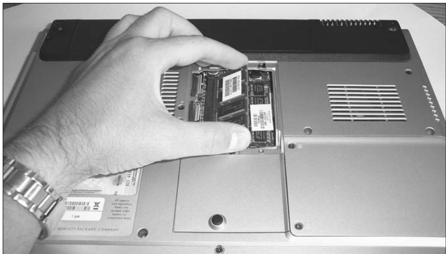
Figure 7-6: Installing a SODIMM into the laptop to add more memory to the laptop.
