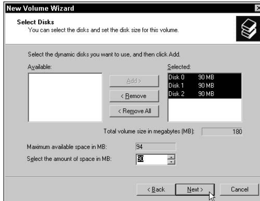
Figure 5-40: Select the disks to be members of the RAID 5 volume and specify the size of the volume.
