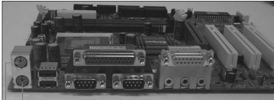
Figure 1-15: Identifying the PS/2 connections used for a keyboard and mouse.
