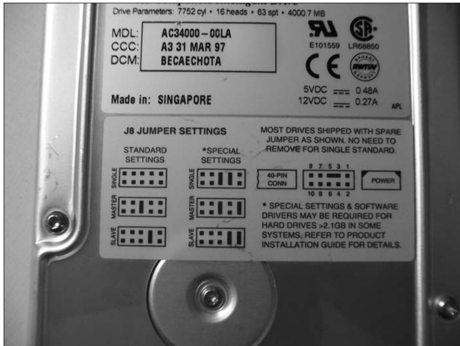
Figure 2-5: Some drives have multiple jumper configurations for the same setting.
