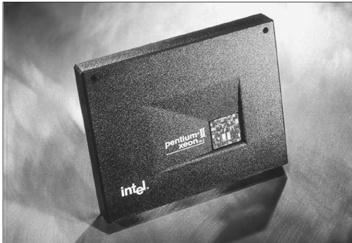
Figure 2-13: The Pentium II Xeon processor was originally delivered in the SEC package.
