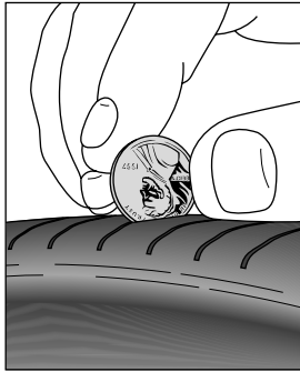
Figure 5-1: The penny test — this tire fails.
