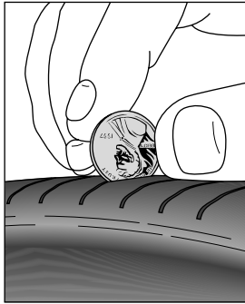
Figure 5-1: The penny test — this tire fails.
