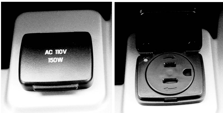
Figure 9-11: A 110-volt outlet in a Ford Escape.
