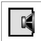
Figure 16-5: A sealed enclosure.
