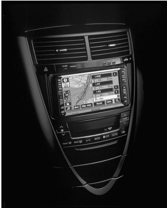
Figure 7-9: The Eclipse AVN5495 has a hard- disc drive that's used for navigation as well as storing music files.
