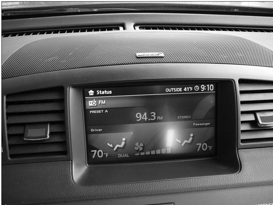
Figure 15-3: A speaker in the center of the dash in an Infiniti M35.
