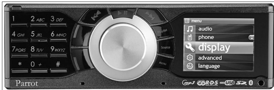
Figure 8-6: Parrot's RK8200 is a car audio head unit with Bluetooth built in.
