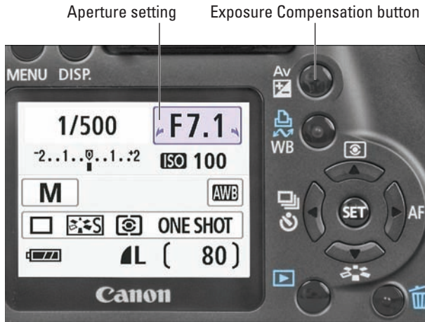
Figure 5-15: To set aperture in M mode, press the Exposure Compensation button as you rotate the Main dial.
