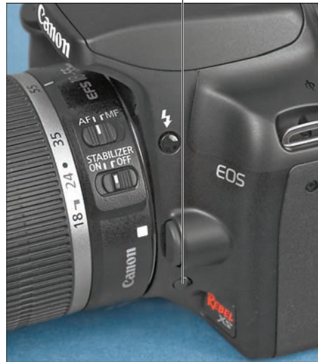
Figure 6-15: Press this button to see how the aperture setting will affect depth of field.
