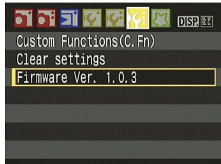
Figure 1-18: To display Setup Menu 3, you must set the Mode dial to an advanced exposure mode.
