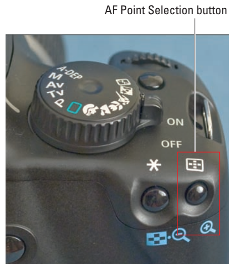
Figure 6-3: Press and release the AF Point Selection button to select an autofocus point.
