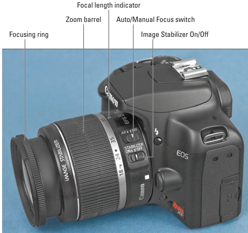
Figure 1-3: Set the focusing switch to MF before turning the manual focus ring.
