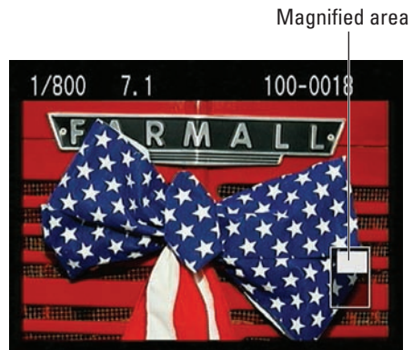
Figure 4-8: Press the cross keys to scroll the display of the magnified image.
