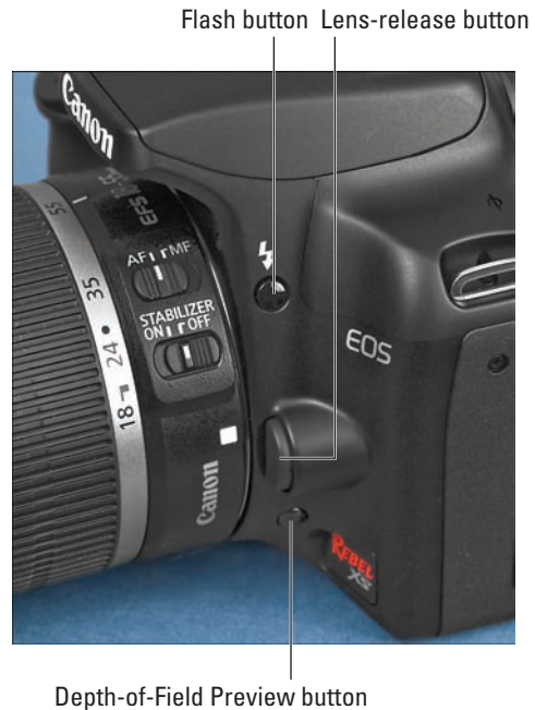
Figure 1-9: Press the Flash button to bring the built-in flash out of hiding.
