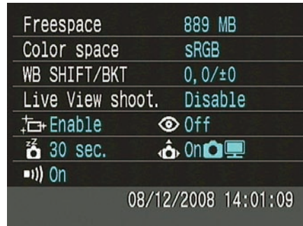
Figure 1-13: Press the DISP button when the menus are active to view this screen.
