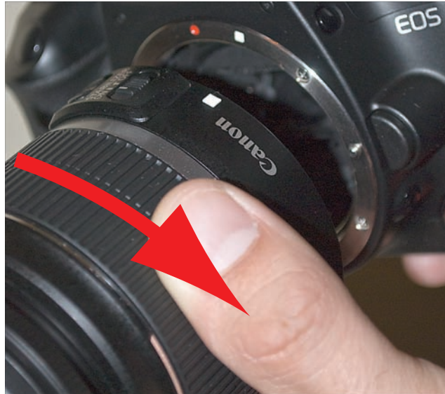
Figure 1-2: Place the lens in the lens mount with the mounting indexes aligned.
