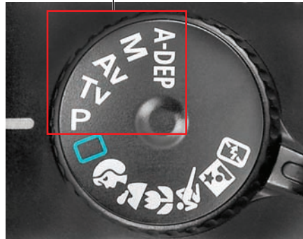
Figure 5-1: You can control exposure and other picture properties only in P, Tv, Av, M, and A-DEP modes.
