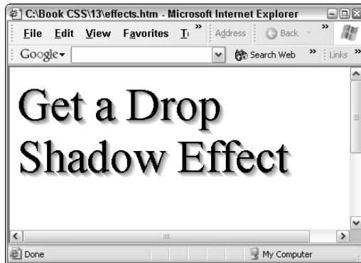
Figure 13-1: Adding shadows is one of 16 static filters you can add to your page elements.
