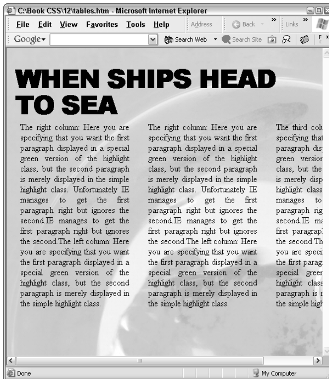
Figure 12-15: When the browser is resized, the columns remain frozen in place.
