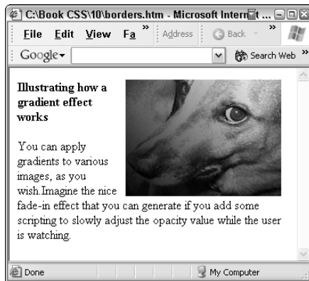
Figure 10-9: Change the float value to right, and you get this effect. Right floats are more often used when inserting photos than left floats.
