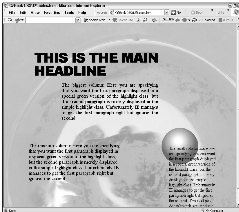
Figure 12-10: Used fixed units if you want your design to remain unaffected by adjusted browser shapes.
