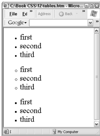
Figure 12-1: The three bulleted (unordered) list styles are dots, circles, and squares.
