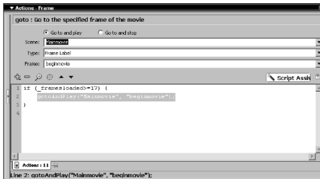
Figure 8-4: The preload loop plays while enough frames download to play the movie without stopping.
