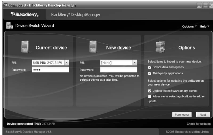
Figure 16-2: Verify that your old BlackBerry is connected to the PC and decide what data to include here.
