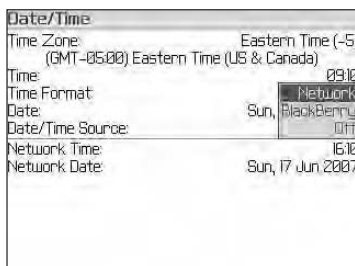
Figure 3-4: Set the time source of your BlackBerry to your network provider's clock.
