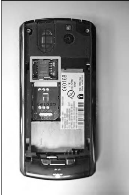
Figure 2-8: The place to insert your microSD slot (upper- right corner) for the BlackBerry Pearl.
