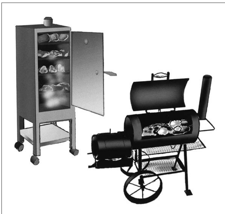
Figure 2-3: On a vertical smoker (left), the meat cooks far above the heat. An offset horizontal smoker separates the fire and the cooking surface.
