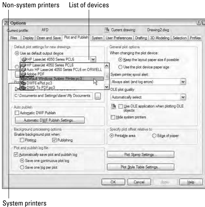
Figure 13-1: System and non-system printer con- figurations.
