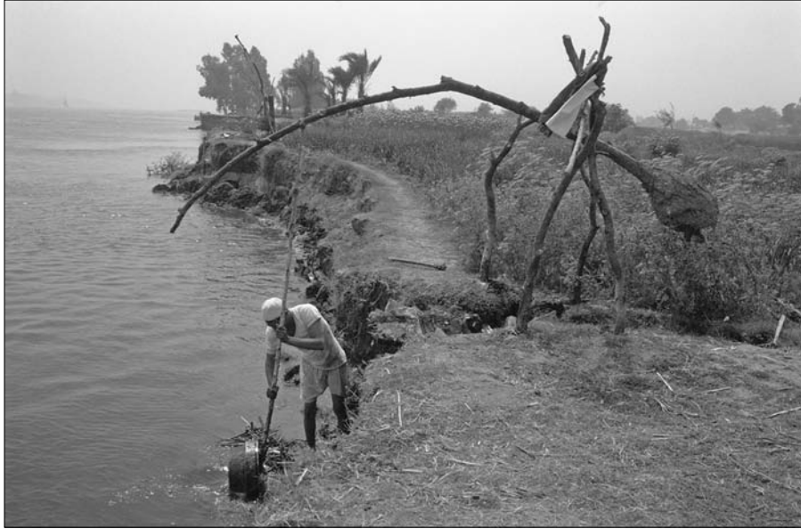
Figure 9-2: Egyptian shaduf irrigation tool in modern times.
