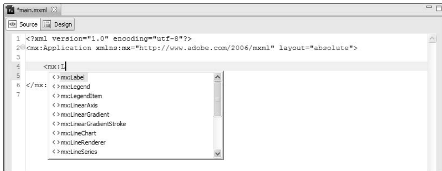
Figure 2-4: The code hinting drop-down list gives you suggestions as you enter code in the code editor.
