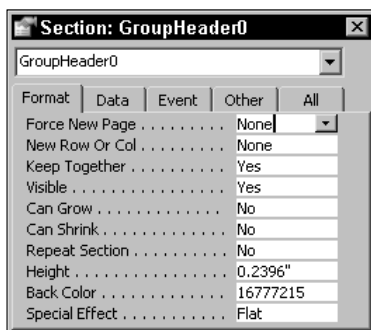
Figure 19-9: Use the Format tab to set group properties that help keep groups together.
