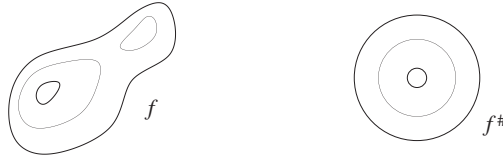
Figure 1.5 A function f on \mathbb{R}^n and its symmetric decreasing rearrangement f^\# . Three level surfaces ( f = c ) are shown. The function in this example is nonnegative, with two local maxima and a saddle point, and vanishes at infinity. By definition, f^\# is the unique radially decreasing, lower semicontinuous function on \mathbb{R}^n that is equidistributed with f .
