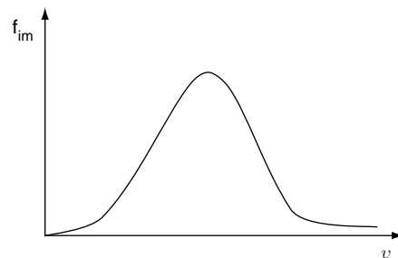
FIGURE 13.3 A relation between the drag force due to impurities on grain boundaries, f_{im}(v) and grain-boundary velocity.
