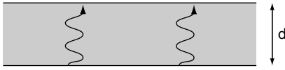
FIGURE 13.5 The geometry of mass transport through a fluid phase at a grain boundary.
