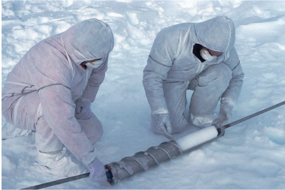
Scientists in Antarctica use a hand drill to take 10-metre ice cores. Chemical analyses of the cores will reveal changes in climate and the composition of the atmosphere.
