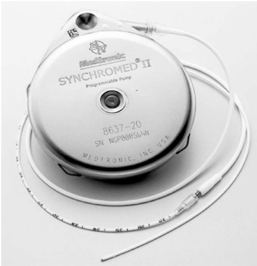
Figure 10.2. A programmable pump, and spinal catheter with centimetre length markings. The refill port is at the centre of the pump body. The aspiration (test) port is in the delivery nacelle. (From Medtronic Ltd., with permission.)
