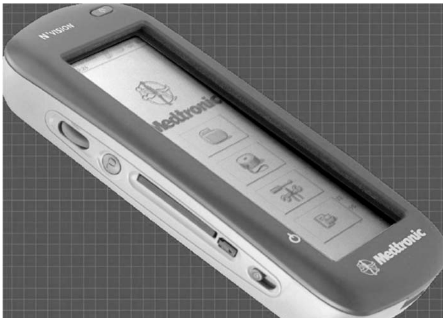
Figure 10.3. Hand-held programmer for use in pump adjustment and refill. (From Medtronic Ltd., with permission.)
