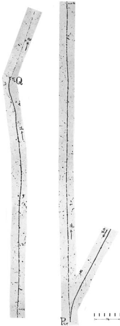
Figure 3.1. A \kappa ( K ) meson stops at P , decaying into a muon and neutrals. The muon decays at Q to an electron and neutrals. The muon track is shown in two long sections. Note the lighter ionization produced by the electron, contrasted with the heavy ionization produced by the muon near the end of its range. The mass of the \kappa was measured by scattering and grain density to be 562 \pm 70 MeV (Ref. 3.4).
