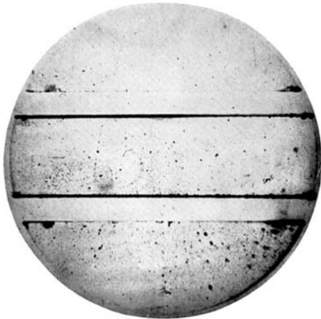
FIG. 4. A positron of about 200 million volts energy ( H\rho = 6.6 \times 10^5 gauss-cm) penetrates the 11 mm lead plate and emerges with about 125 million volts energy ( H\rho = 4.2 \times 10^5 gauss-cm). The assumption that the tracks represent a proton traversing the lead plate is inconsistent with the observed curvatures. The energies would then be, respectively, about 20 million and 8 million volts above and below the lead, energies too low to permit the proton to have a range sufficient to penetrate a plate of lead of 11 mm thickness.
