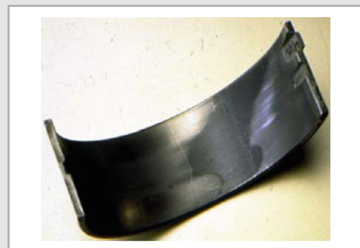
Fig. 8-54 Abrasive wear in a three-layer bearing shell
