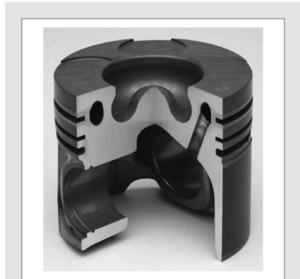
Fig. 8-62 Cooling gallery piston with cooled ring carrier
