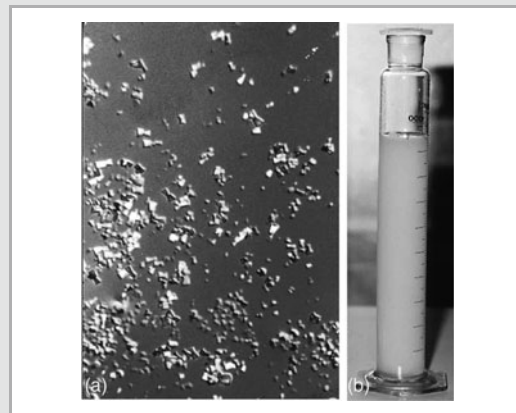
Fig. 4-10 Diesel fuel with flow improvers and wax anti-settling additives at -22^{\circ}\text{C} : No paraffin crystal sedimentation
