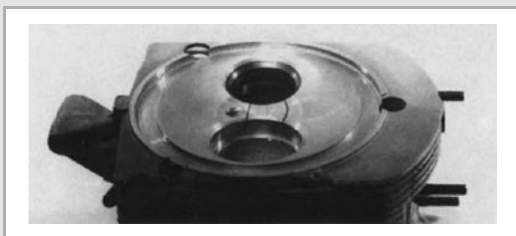
Fig. 9-17 Steel plates cast in valve bridges to prevent valve bridge cracks in the cylinder head of an air-cooled diesel engine (Deutz AG FL 513)
