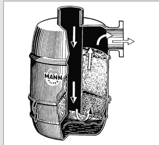
Fig. 13-6 Oil wetted air bath cleaner for diesel engines
