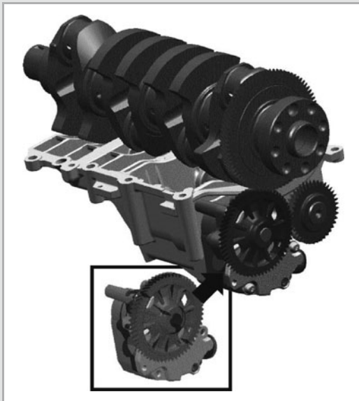
Fig. 17-6 Balance shaft unit for a four cylinder engine
