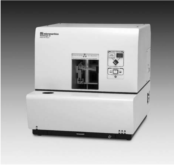
FIG. 21-19 The Sedigraph III 5120 Particle Size Analysis System determines particle size from velocity measurements by applying Stokes' law under the known conditions of liquid density and viscosity and particle density. Settling velocity is determined at each relative mass measurement from knowledge of the distance the X-ray beam is from the top of the sample cell and the time at which the mass measurement was taken. It uses a narrow, horizontally collimated beam of X-rays to measure directly the relative mass concentration of particles in the liquid medium.
