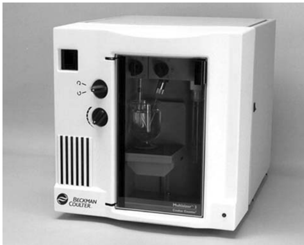
FIG. 21-17 Multisizer™ 3 COULTER COUNTER® from Beckman Coulter, Inc., uses the electrical sensing zone method.
