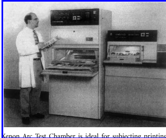
FIGURE 16.3 The Q-Sun Xenon Arc Test Chamber is ideal for subjecting printing inks and substrates to full-spectrum sunlight.
