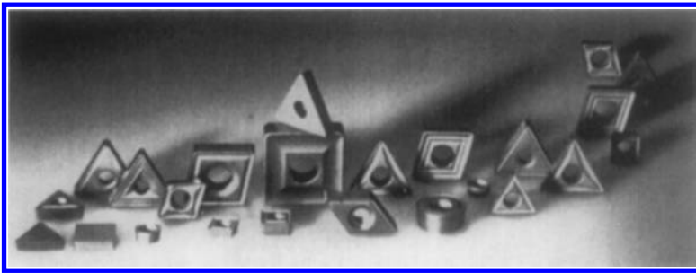
FIGURE 35.5 Photography showing cemented tungsten carbide cutting tool inserts coated with TiC and TiN coating in a conventional CVD process. These coatings impart improved wear resistance to the carbide tools, allowing them to run at higher speeds and chip loads in the machining of various materials.
