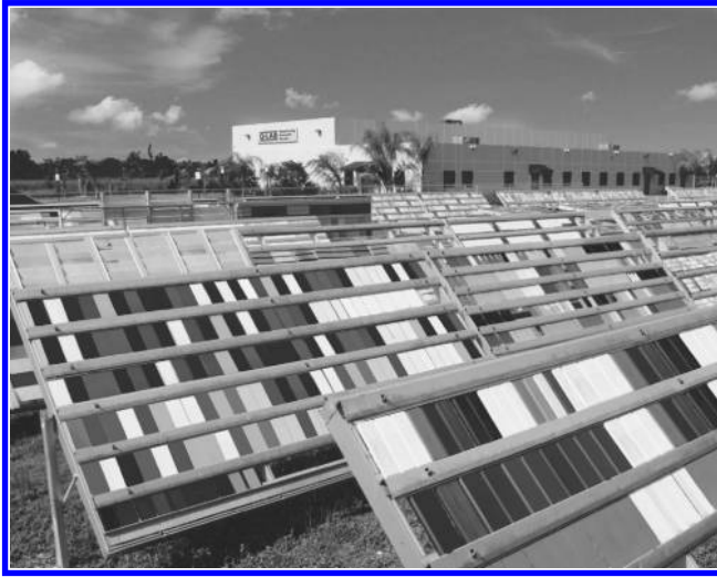
FIGURE 118.1 Q-Lab weathering research service test facilities research center in Florida and Arizona performed fade resistance testing of lithographic inks in extreme environments.
