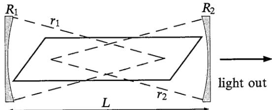
Cavity stability condition  $0 \leq \left(1 - \frac{L}{r_1}\right) \left(1 - \frac{L}{r_2}\right) \leq 1 \quad (8.123)$
