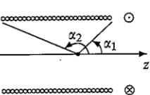
The axis,  $z$ , of a straight solenoid,  $n$  turns per unit length, current  $I$
