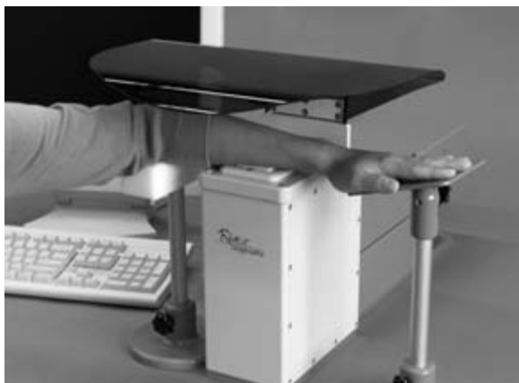
Figure 1 The river diagnostics model 3510 skin composition analyzer is the first Raman instrument optimized for in vivo analysis of skin.
