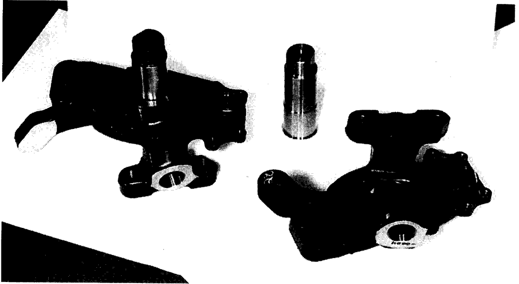
Figure 5.3 Irregularly shaped parts to be selectively induction hardened.
