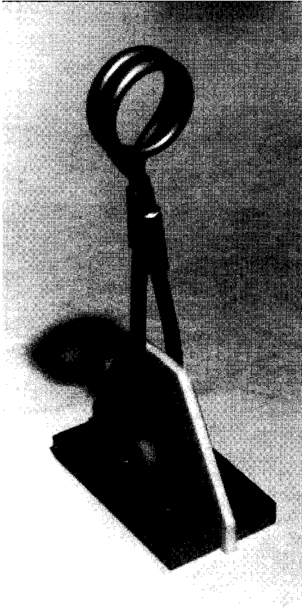
Figure 6.8 Brazing inductors are often simple in design.
