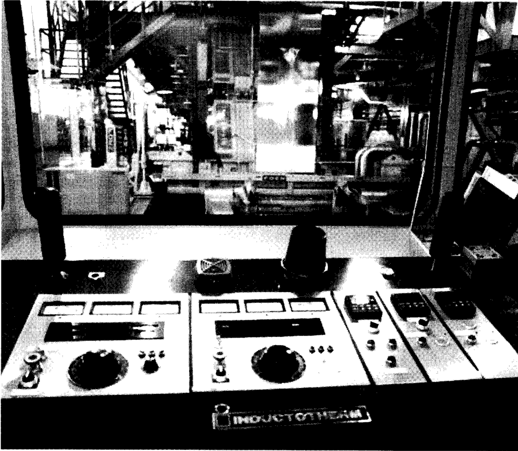
Figure 2.48 Induction strip galvanizing line. (Built in cooperation between INDUCTOHEAT, Inc. and Inductotherm Corp.)
