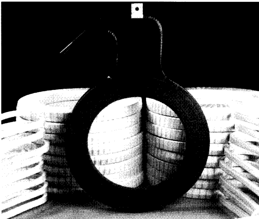
Figure 7.27 Multilayer disc-pair copper winding. (Courtesy of Inductoheat Banyard Ltd., UK.)
