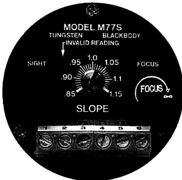
Figure 4.8 Two-color ratio thermometer. (Courtesy of Mikron Instrument Company, Inc.)
