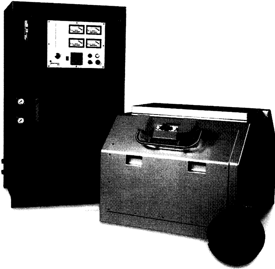
Figure 6.28 Induction die heater. (Courtesy of Inductoheat Banyard, UK.)
