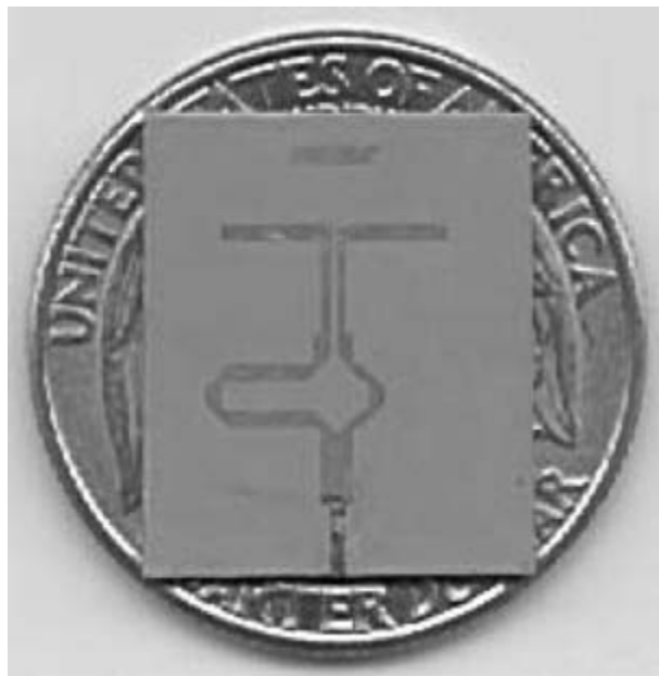
FIGURE 11.20 Layout of Quasi-Yagi Antenna (Left) and Photograph of X-Band Prototype (Right)
