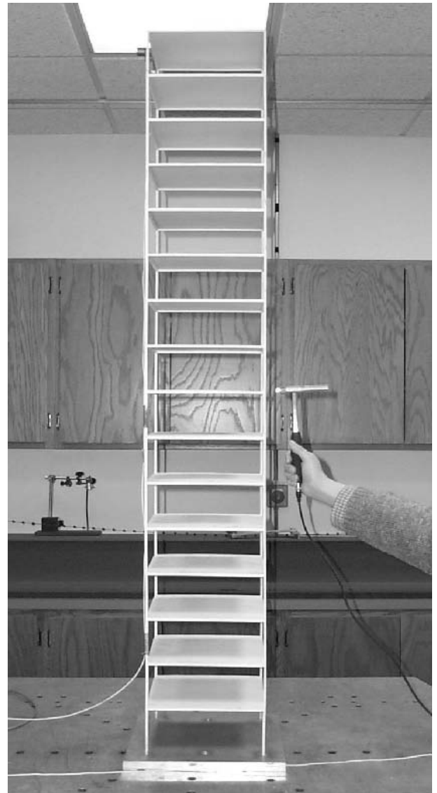
FIGURE 6.2 Picture of the 16-Story Structure
