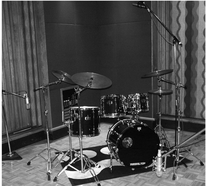
Figure 81 Three Mic Setup— M149 on Left, U47 in Front, and Royer R-121 Overhead
