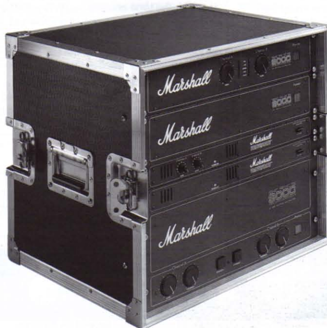
Rack-mounting MESA/Boogie and Marshall, among others, offer rack mounting versions of their equipment. MESA/Boogie offer the option of a "retro kit" to allow combo amps to be converted for rack mounting.
