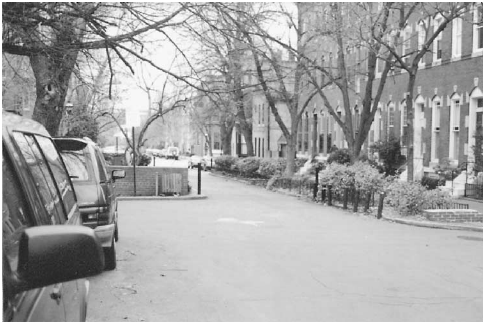
Figure 8.12 Bollards and plantings used in a city neighborhood separate public from private space and signal community activity and surveillance.
