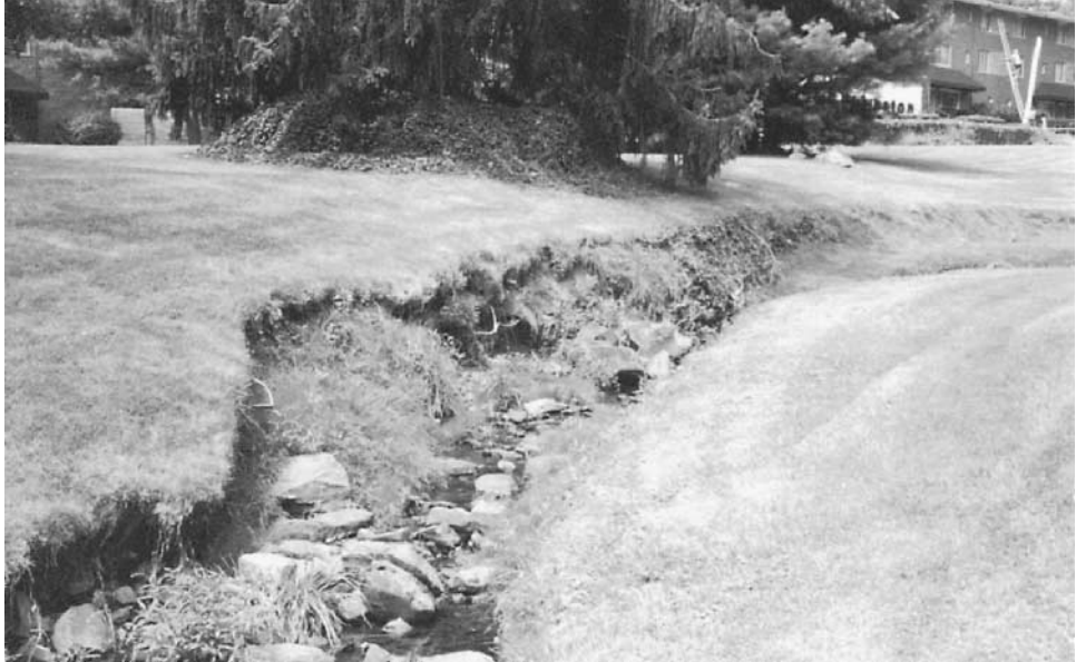
Figure 7.15 Photograph of an urban stream in which the bank is retreating from the stream.
