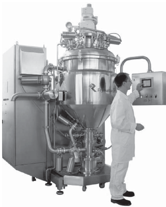
FIGURE 3 Vacuum processing machine used for preparation of gels. (Courtesy of FrymaKoruma-Rheinfelden, Switzerland.)
