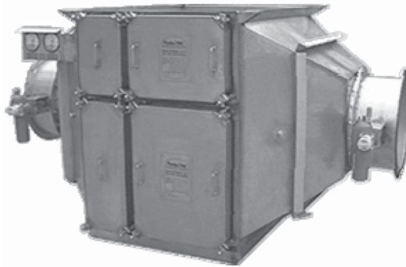
FIGURE 16 The “bag-in-bag-out” filter unit contains a HEPA filter and permits personnel to change the filter without coming into contact with possibly hazardous materials that may have been filtered from the air. (Courtesy of Flanders Filters Inc.)
