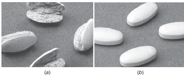
FIGURE 28 Tablets coated with (a) conventional hypromellose and (b) Sepifilm LP 770 white.
