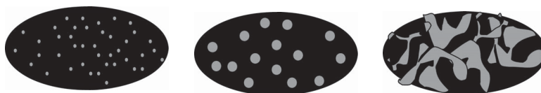
FIGURE 3 Schematic pictures of insoluble matrix systems. Left: Drug (light gray) molecularly dissolved in carrier material (black); middle: drug particles dispersed in carrier material; right: drug particles dispersed in carrier material at higher drug loading, leading to continuous network of drug.
