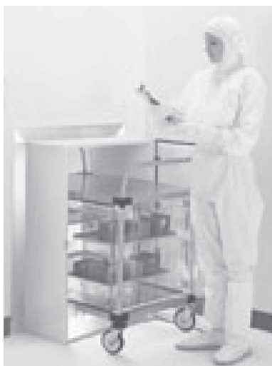
FIGURE 3 Cart pass-through enabling larger amounts and sizes of items to be transported. Note that the cart shown is not to be taken from the clean room. Typically a physical barrier is incorporated into the cart pass-through design. (Courtesy of Terra Universal.)
