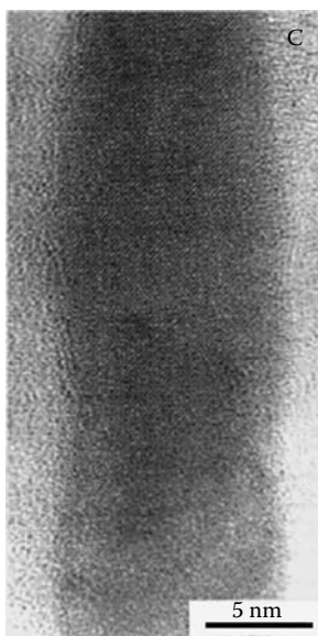
FIGURE 9.20 TEM image of 8-nm cobalt nanowire. (Courtesy of Dr. Yi Liu.)
