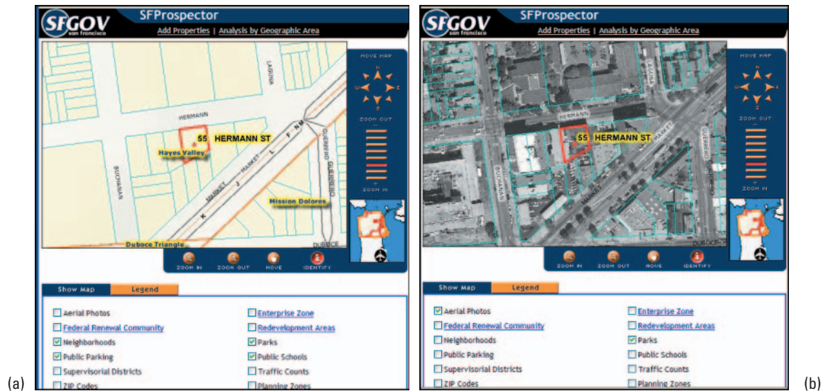
FIGURE 14-16 Different themes on different layers: (a) neighborhood and (b) aerial photo layers. 19
