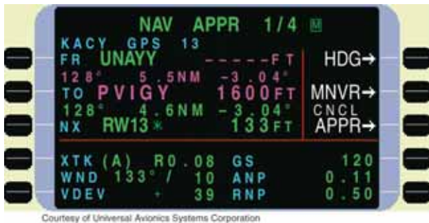
Figure 1-15. FMS Control Display Unit. This depicts an aircraft established on the Atlantic City, NJ, RNAV (GPS) Rwy 13 instrument approach procedure at the Atlantic City International Airport, KACY. The aircraft is positioned at the intermediate fix UNAYY inbound on the 128 degree magnetic course, 5.5 nautical miles from PVIGY, the final approach fix.
