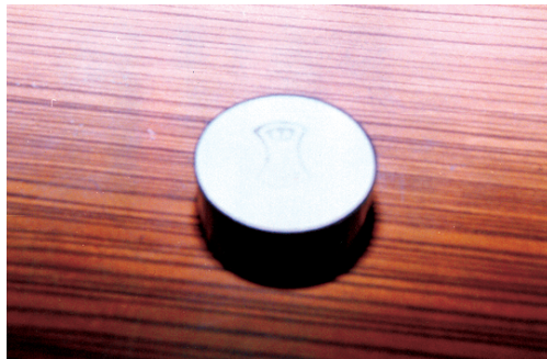
Fig. 8.1: Metal oxide surge arrester block
