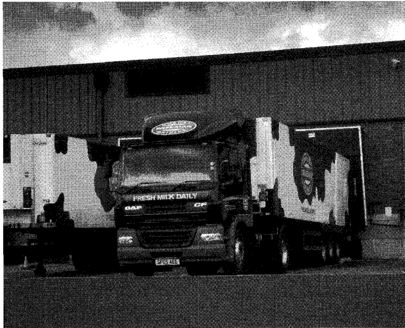
Figure 23.8 An articulated combination featuring a box trailer, which in this case is refrigerated (courtesy of Daf Trucks)
