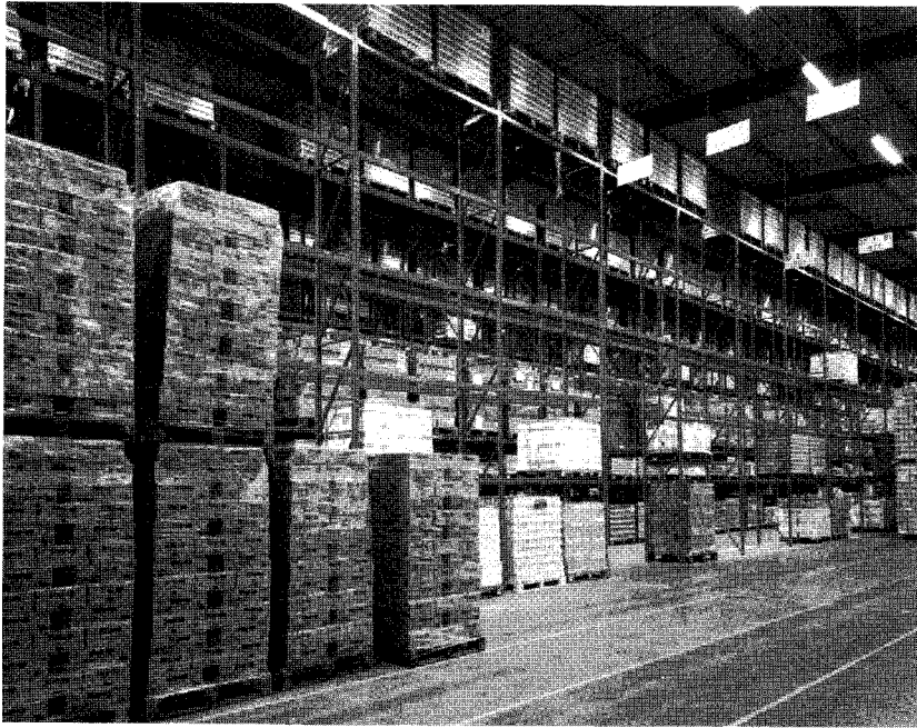
Figure 15.5 Block stacking in foreground, with adjustable pallet racking behind ( courtesy of Redirack)
