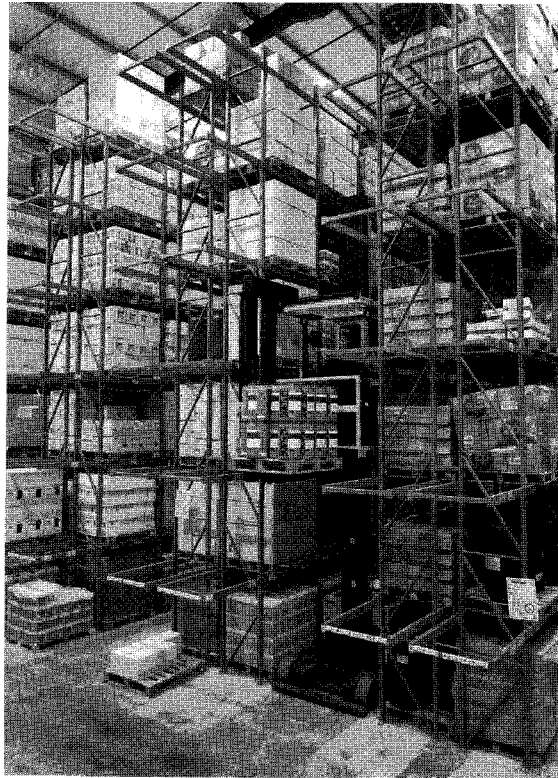
Figure 15.8 Narrow-aisle racking (courtesy of Redirack)
