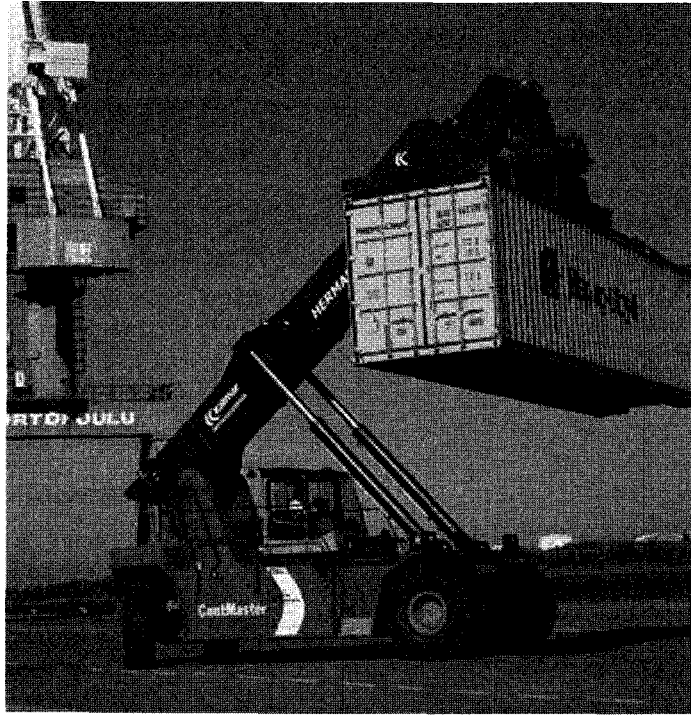
Figure 22.3 Reach stacker handling an ISO container
