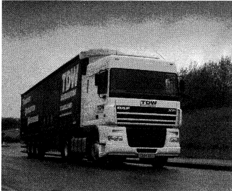
Figure 23.1 Articulated vehicle made up of a tractor and semi-trailer (courtesy of Daf Trucks)
