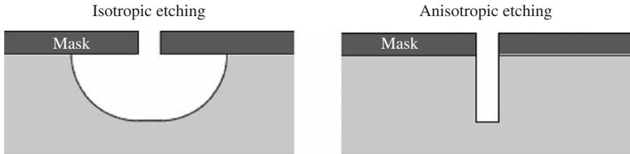
FIGURE 24.4 Isotropic and anisotropic etching.
