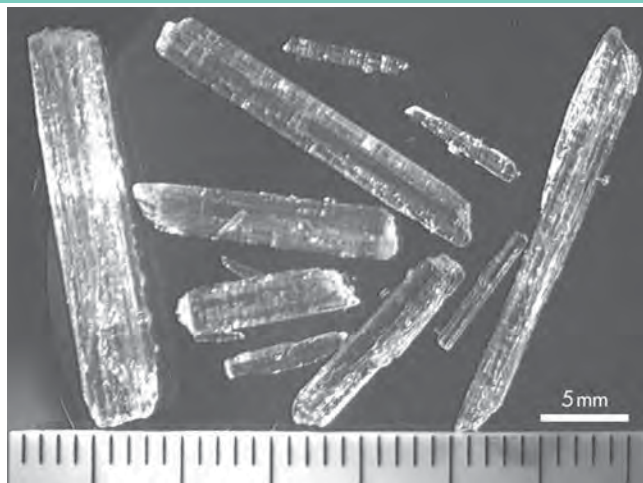
Figure 1: Photomicrograph of large DL-menthol crystals; magnification 7 \times . Manufacturer: Charkit Chemical Corp., USA.
