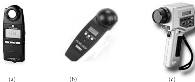
FIGURE 32 Handheld lighting measurement instruments. (a) Simple Luxmeter; (b) Luxmeter (from Labsphere) with an integrating sphere as a diffuser; and (c) luminance meter (from Konica Minolta).
