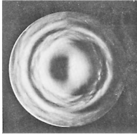
FIGURE 2 An optical surface being examined by the Foucault test. (From Ojeda-Castañeda. 3 )
