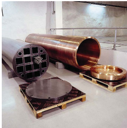
Figure 70 An example of spent fuel packaging: the SKB Swedish concept, with a thick-walled copper canister (photo SKB) (Papp 1998a)
