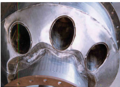
■ Figure 232 Prediction of buckled mode shape by CAST3M
