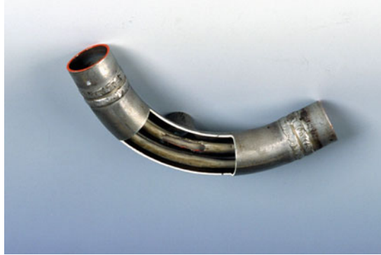
■ Figure 16 Hydrogen-meter based on Ni diffusion
