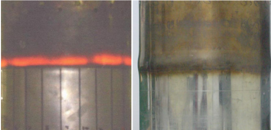
■ Figure 200 Symmetric bulging of shell subjected to sharp axial thermal gradient
