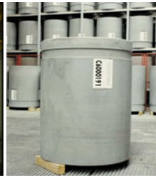
Technological waste enrobed in concrete
