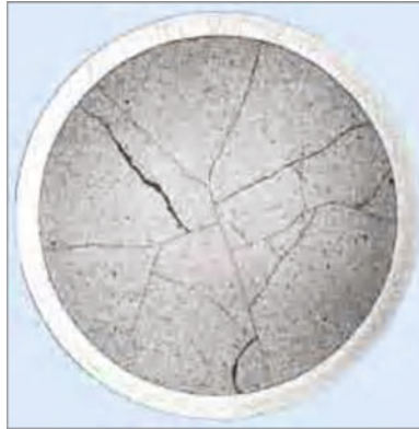
Figure 73 Radial macrograph of a spent fuel pellet
