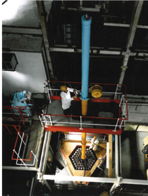
Figure 147 Operating the CEA 106 E rig in Cadarache (handling test)
