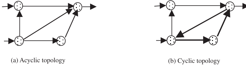
1.2 Illustration of (a) an acyclic graph and (b) a cyclic graph. The cycle in (b) is emphasized with thick lines.
