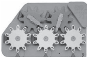
FIGURE 20.2. The pascaline Zero + 1 (representing 620).
