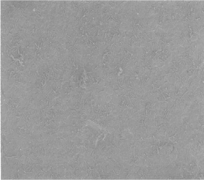
Figure 18.1. Biofilm formation after 1–2 h on stainless steel, \times 1000 magnification.
