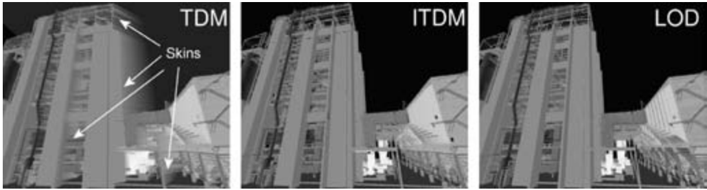
Figure 20.9 Comparison of Incremental Textured Depth-Meshes (ITDMs) [96] with regular TDMs and geometric levels of detail (LODs) on a 12.5M polygon power-plant model. ITDMs generate images almost as well as do static LODs, and at a frame rate 9 times faster. Moreover, ITDMs do not show the skin artifacts common in TDMs. The TDMs and ITDMs are used as a simplification of the far geometry. Copyright © 2003 Association for Computing Machinery, Inc. (See also color insert.)
