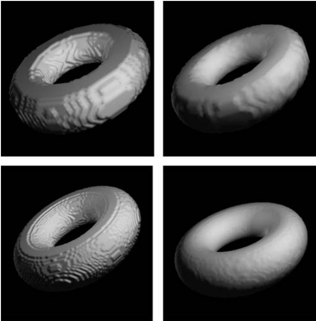
Figure 6.12 (Left) Binary input volumes. (Right) Results of surface estimation. (Top) Lower-resolution torus. (Bottom) Higher-resolution torus.
