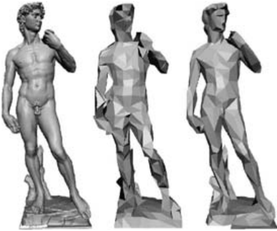
Figure 20.8 Hybrid regular/adaptive simplification process for the David model (Stanford’s Digital Michelangelo Project). (Left) Original model (8 million triangles). (Middle) Simplified using regular cell clustering (1,157 triangles). (Right) Simplified using multiphase approach to cell clustering followed by priority queue–driven edge collapses (1,000 triangles) [34]. Copyright © 2002 IEEE.
