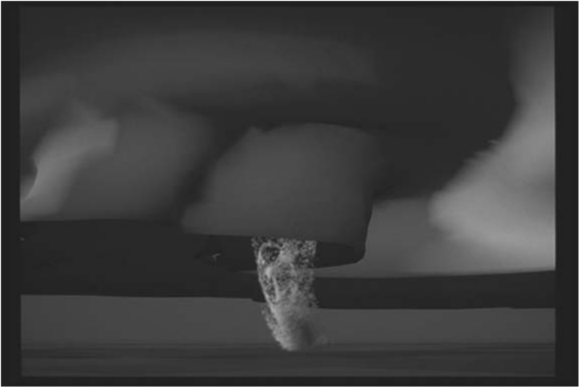
Figure 44.9 Visualization of a developing tornado revealed through the use of thousands of circulating particles. (See also color insert.)
