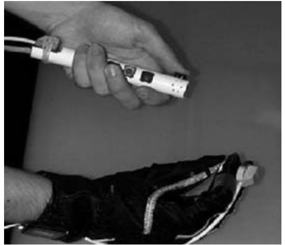
Figure 23.11 Button stick (top) and glove with finger contacts (bottom): two modes for 6 DoF interaction. (See also color insert.)
