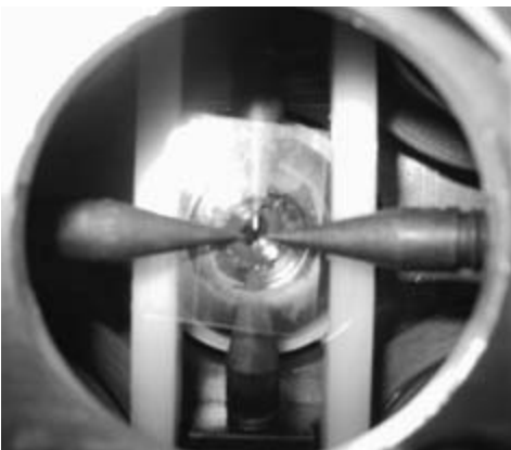
Figure 46.15 Photograph of four magnetic poles in a 3DFM surrounding a specimen mounted between two cover slips. (See also color insert.)
