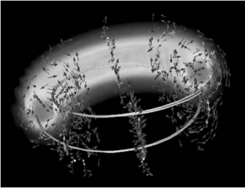
Figure 31.9 A simulation of an experiment inside a Tokamak Fusion Reactor, visualized with the SCIRun Fusion package. This is frame one of two from a time sequence showing the stochastic nature of the real-space magnetic field lines. A comparison of the two frames shows that the magnetic field lines start to diverge earlier as time progresses. The field lines are overlaid in a volume rendering of the pressure field, which provides visual cues to the location while rendering the plasma velocity-vector field. Image provided by Dr. Allen Sanderson and the National Fusion Collaboratory with support from the US Department of Energy SciDAC initiative. (See also color insert.)
