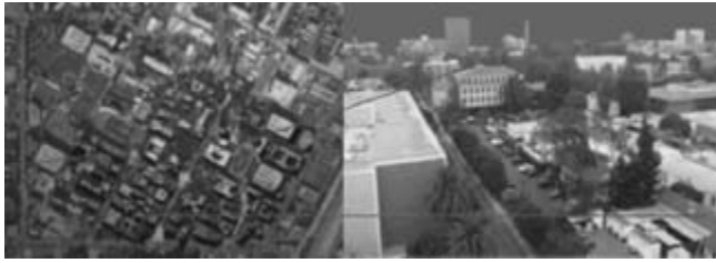
Figure 23.2 High-resolution aerial imagery merged with georeferenced models automatically extracted from LIDAR data [66]. (See also color insert.)
