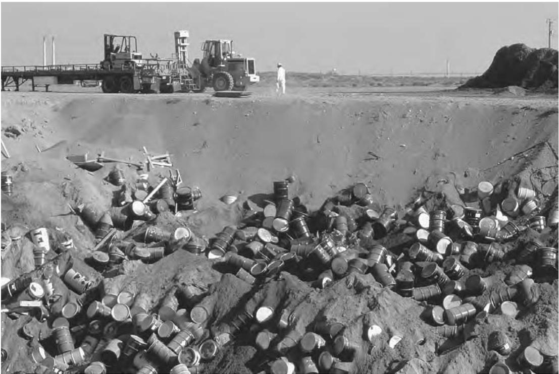
*Steel drums full of class-A low-level radioactive waste buried in a large trench at the Hanford Nuclear Reservation. (Roger Ressmeyer/Corbis)*
