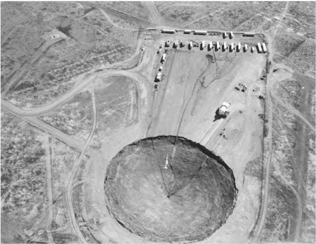
*Monitoring station and subsidence crater formed by an underground nuclear test at the Nevada Test Site (Huron King test, June 1980) (DTRA)*
