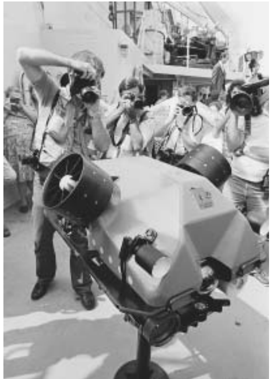
Jason Junior, a submersible, highly maneuverable camera, allowed from Woods Hole Oceanographic Institute to explore the wreck of the R.M.S. Titanic . © Bettmann/Corbis. Reproduced by permission.
