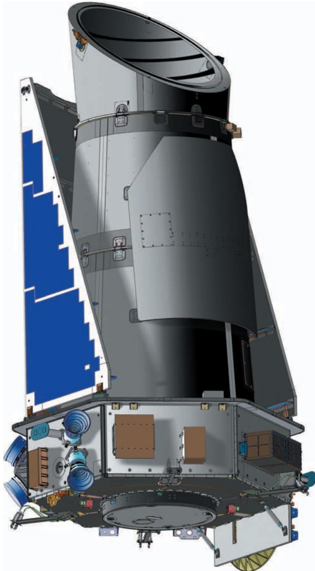
FIGURE 14 Artist conception of the Kepler photometer and spacecraft. A 1 m Schmidt telescope will observe a large section of the sky in the constellation Cygnus continually for over 4 years to detect transits of Earth-sized planets in Earth-like orbits across the disks of solar-type stars. Launch is scheduled for late 2008. (Image courtesy NASA Kepler project.)
