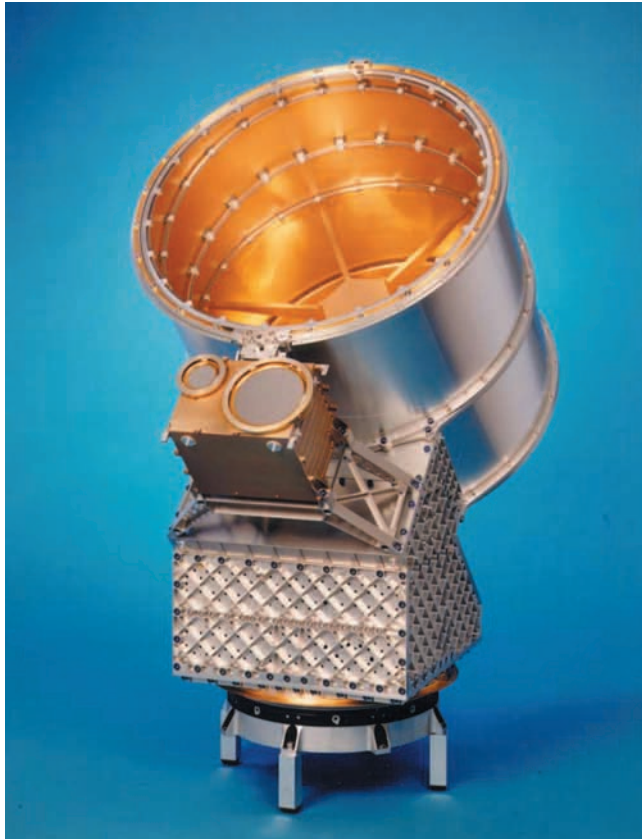
FIGURE 7 The Cassini cosmic dust analyzer consists of two types of dust detectors—the high rate detector (HRD) and the dust analyzer (DA). The cylindrical DA (upper center) has a diameter of 43 cm. The bottom of the sensor contains the hemispherical impact target; in the center are charge-collecting electrodes and the multiplier for measurement of the mass impact spectrum. Two entrance grids sense the electric charge of incoming dust grains. The detector records impacts of submicrometer- and micrometer-sized dust particles above an impact speed of 1 km/s. HRD consists of two circular film detectors that record impacts of micrometer-sized dust particles at a rate of 10,000 per second. The detectors are carried by the electronics box that is mounted on top of a turntable bolted to the spacecraft.
