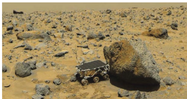
FIGURE 18 Color mosaic of Sojourner with APXS instrument measuring the chemical composition of the rock Yogi. Note dusty surface darkened by the rover wheels. Brighter toned soil in the wheel tracks is cemented soil or duricrust. Note tabular rock on the left horizon, called Couch, and other tabular and partially rounded boulders as expected if deposited by catastrophic floods.
