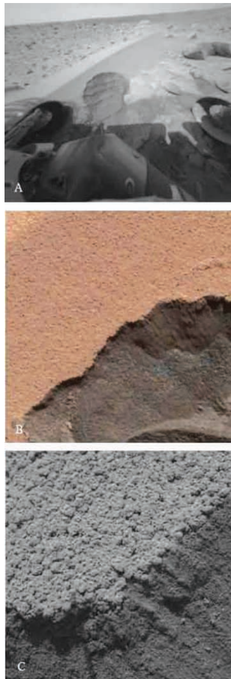
FIGURE 17 Large ripple called Serpent that was studied by Spirit on the cratered plains. (A) A Hazard Camera image showing the rover front wheels and the tracks produced by a wheel wiggle maneuver to section the drift. (B) Color image of the dusty (reddish) surface and darker more poorly sorted interior. (C) MI image of the brighter (dust cover) granule-rich surface (millimeter-sized particles) and poorly sorted, but generally finer grained, basaltic sand interior. The dusty, granule-rich surface indicates the eolian feature is an inactive (dust cover) ripple formed by the saltation induced creep of granules, which are left as a lag.
