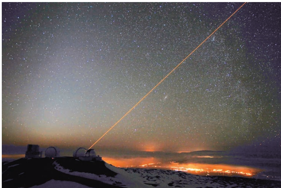
FIGURE 14 Sodium laser guide star in use at Keck II. The laser operates at a wavelength of 5890 Angstroms (0.589 micrometers), and the laser light is propagated through a smaller telescope attached to the Keck telescope. It excites sodium atoms in a layer in the Earth's atmosphere at an altitude of 90 km. The sodium atoms emit light at the same wavelength as the laser and this is viewed as an artificial star by the telescope. (This is a long exposure photograph. The laser guide star is barely visible with the naked eye from this angle. The lights of the island of Hawaii are below the clouds. (Courtesy of Jean-Charles Cuillandre.)
