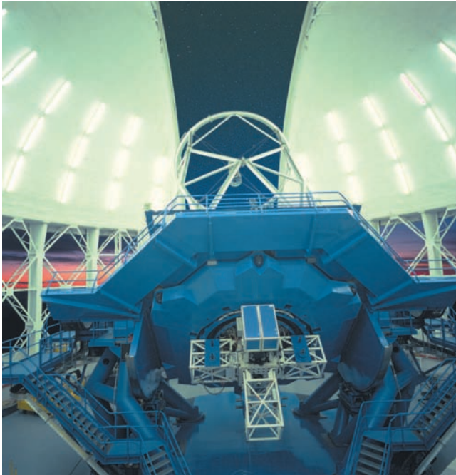
FIGURE 6b 8-m Gemini South telescope. Instruments are mounted on the back of the telescope. These instruments are on the telescope all of the time so that instrument changes can be made very quickly. The dome has vents to allow flushing of the dome by the night air. This allows the telescope and dome to quickly reach equilibrium with the air temperature. (Courtesy of Gemini Observatory/AURA)
