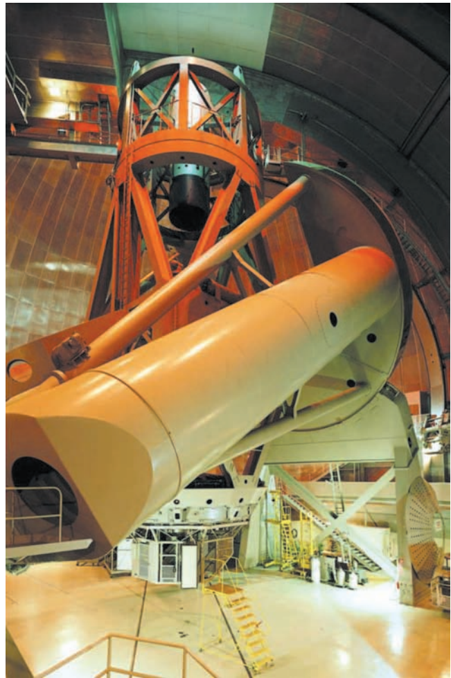
FIGURE 6a Hale 5.1-m telescope. The last large telescope to be built in the “classical style” with an equatorial mount, a culmination of about 280 years of development of the reflecting telescope. © 2005 Gigapxl Project
