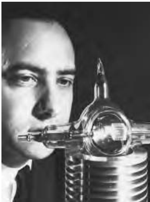
Theodore H. Maiman studies a ruby crystal in the shape of a cube in the first laser. (Bettmann/Corbis)
