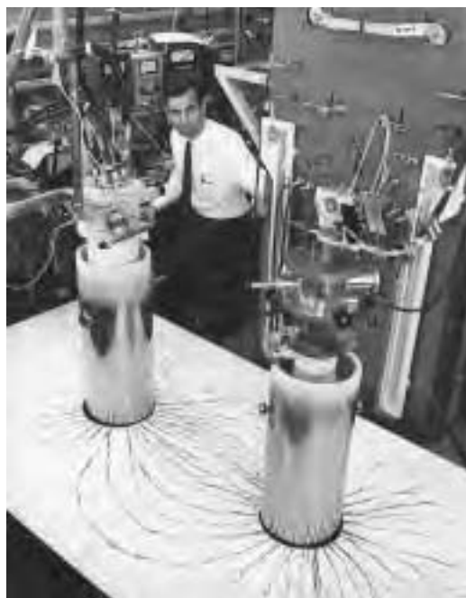
Two magnets based on superconducting technology demonstrate the lines of magnetic force with iron nails. (Bettmann / Corbis)
