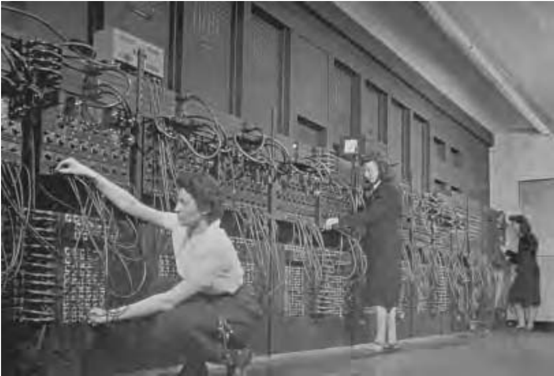
Computer operators program ENIAC, the first successful electronic digital computer, by plugging and unplugging cables and adjusting switches. (Corbis)
