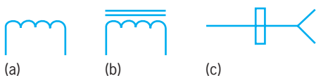
Graphic symbols for chokes or inductors in electric circuits. (a) Choke or inductor with air core. (b) Choke or inductor with magnetic core. (c) Waveguide choke.
