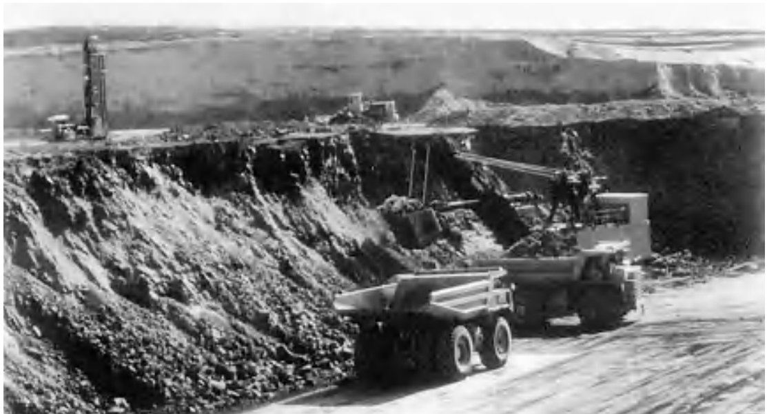
Fig. 5. Power shovel loading coal trucks.
