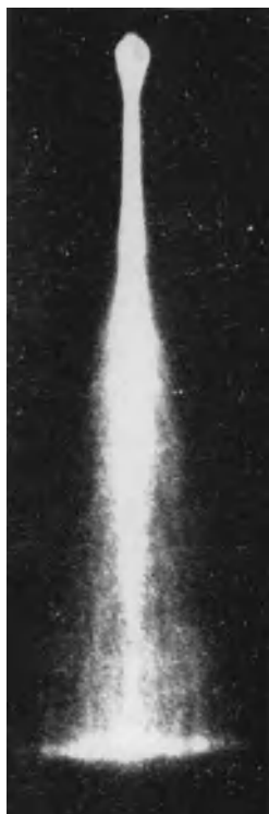
Breakdown streamers in positive-point corona crossing from positive point to cathode below. (From L. B. Loeb, Fundamental Processes of Electrical Discharge in Gases , Wiley, 1939)
