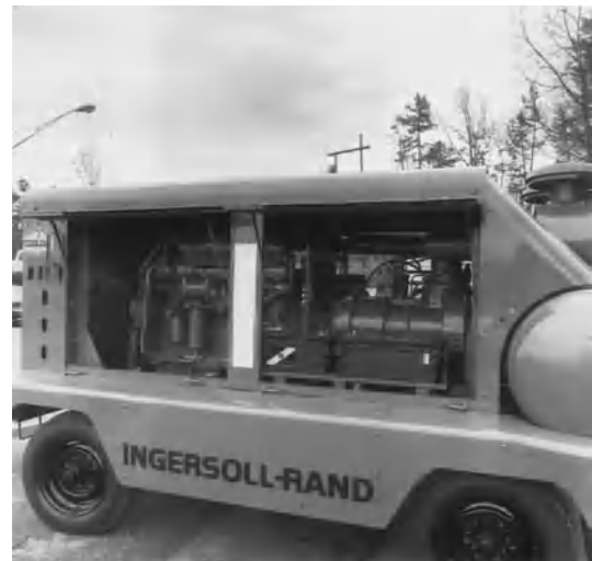
Fig. 1. Mobile air compressor unit which is driven by engine in the forward compartment. (Ingersoll-Rand)
