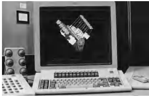
Fig. 2. Solid modeling and simulation on a mainframe via a CAE workstation.
