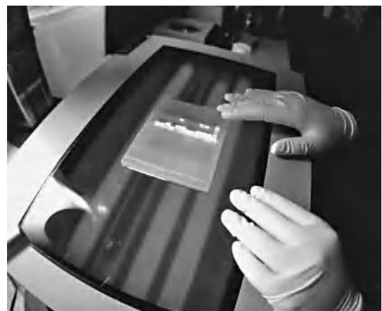
Fig. 6. Examination of an agarose gel with an ultraviolet light source to identify diagnostic fragments of DNA (orange-yellow fluorescent bands in the gel).
