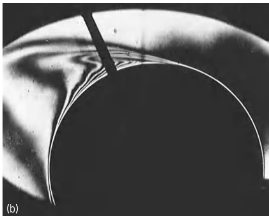
Fig. 3. Interference photographs of isotherms around a heated horizontal cylinder 4 in. (10 cm) in diameter. (a) Cylinder in still air. The outer broad fringe indicates the approximate edge of the boundary layer, which is about \frac{3}{4} in. (2 cm). (b) Cylinder normal to a 33-ft/s (10-m/s) airstream. The boundary layer on the forward half of the cylinder is so thin that the isotherms cannot be resolved. (Courtesy of D. L. Doughty and W. H. Giedt)
