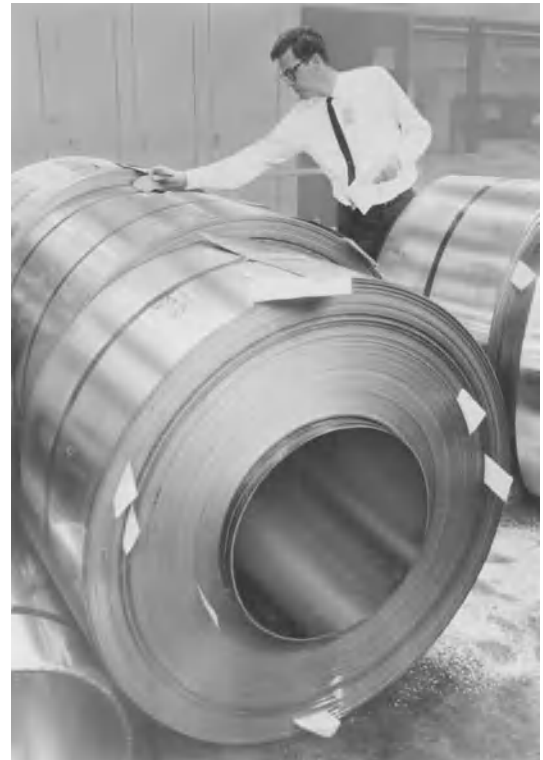
Fig. 1. Rolls of copper clad with copper-nickel facing for minting composite coins.
