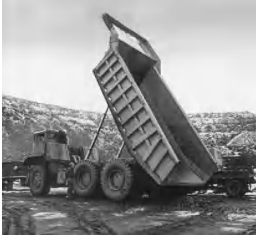
Fig. 6. A 100-ton (90-metric-ton) rear-dump truck.
