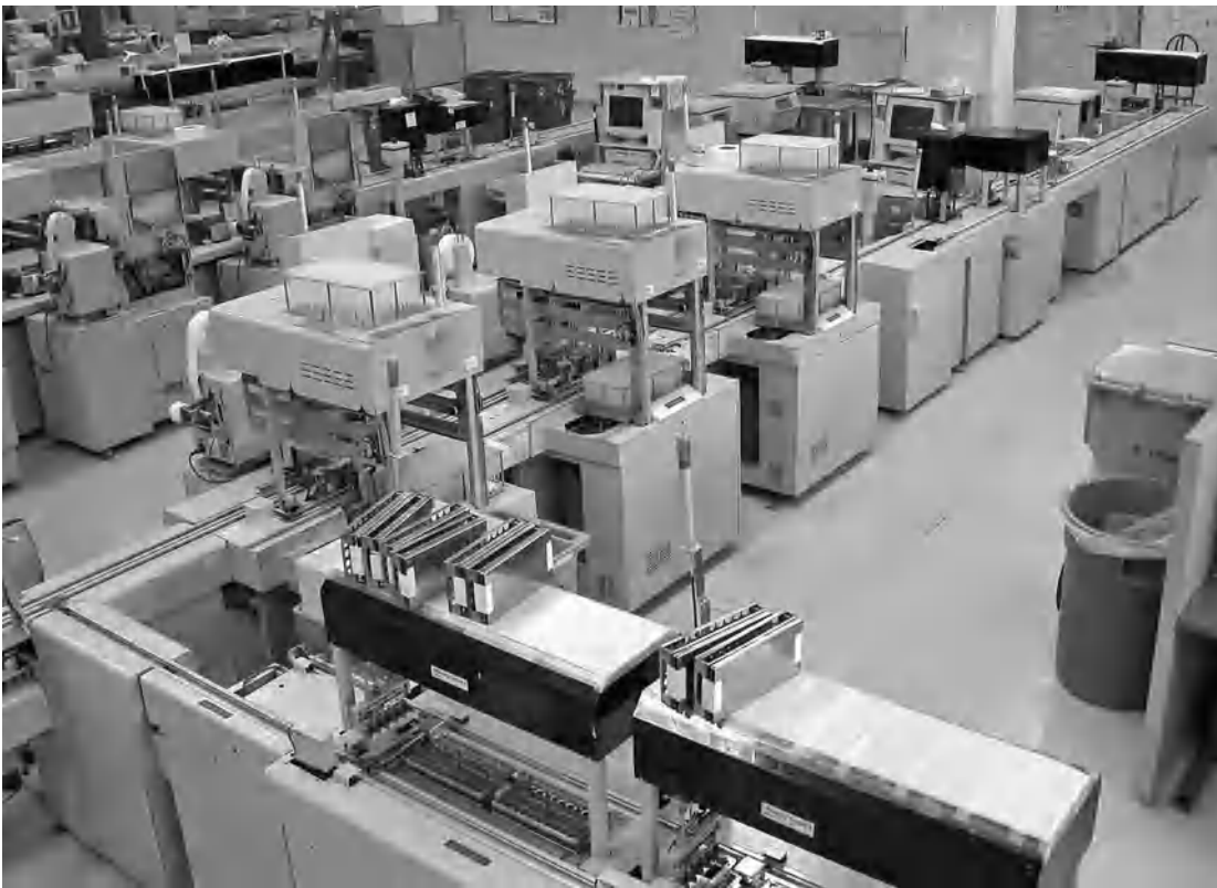
Fig. 2. Overview of a 2005 automated chemical analysis system. Specimen racks are placed on a movable track that moves sequentially through sampling, read-out, and reporting stations in the course of multitest analyses.
