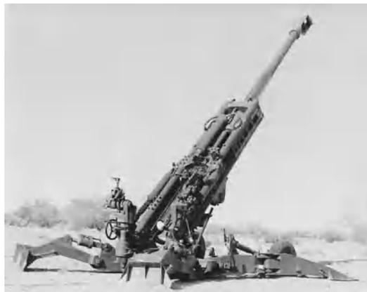
Fig. 3. XM777 lightweight 155-mm towed howitzer. (U.S. Army)
