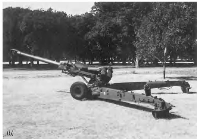
Fig. 1. 155-mm howitzers. (a) M109A6 Paladin self-propelled howitzer (BMY Combat Systems). (b) M198 towed howitzer (U.S. Army).
