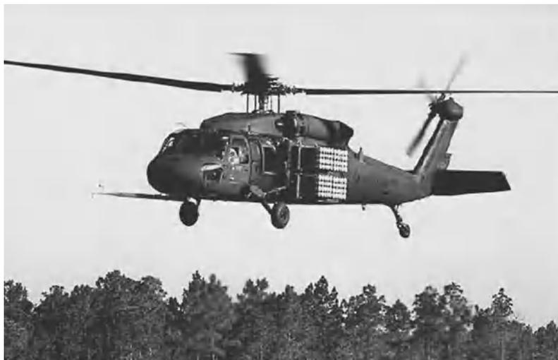
Fig. 15. Volcano modular mine-dispensing system (helicopter-mounted). (U.S. Army)
