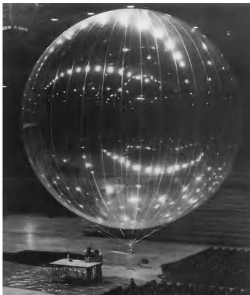
Fig. 2. Superpressure balloon. (Raven Industries)
