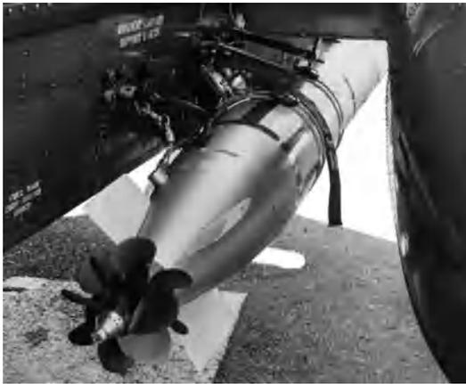
Fig. 4. Mark 46 lightweight homing torpedo aboard a helicopter. (U.S. Navy)
