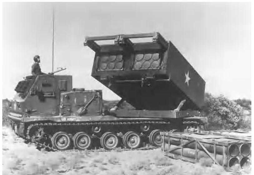
Fig. 4. Multiple-launch rocket system (MLRS). (Vought Corp.)
