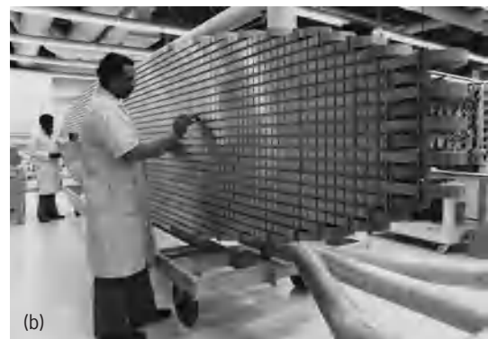
Fig. 2. Air Force AWACS (Airborne Warning and Control System) in use. (a) AN/APY-1 rotodome installed. (b) Precision-array antenna of the AN/APY-1. (Northrop/Grumman Corp.)
