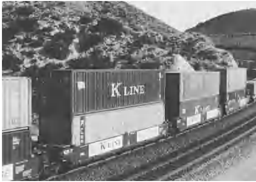
Fig. 3. Articulated double-stack container train, showing single four-wheel truck under one end each of two adjacent cars, and containers stacked two high. (Gunderson, Inc.)
