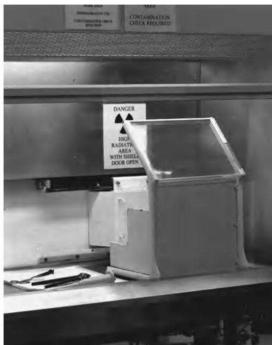
Fig. 2. Fume hood set up with portable shielding and small tongs for working with low-level beta- and gamma-emitting isotopes. (Brookhaven National Laboratory)
