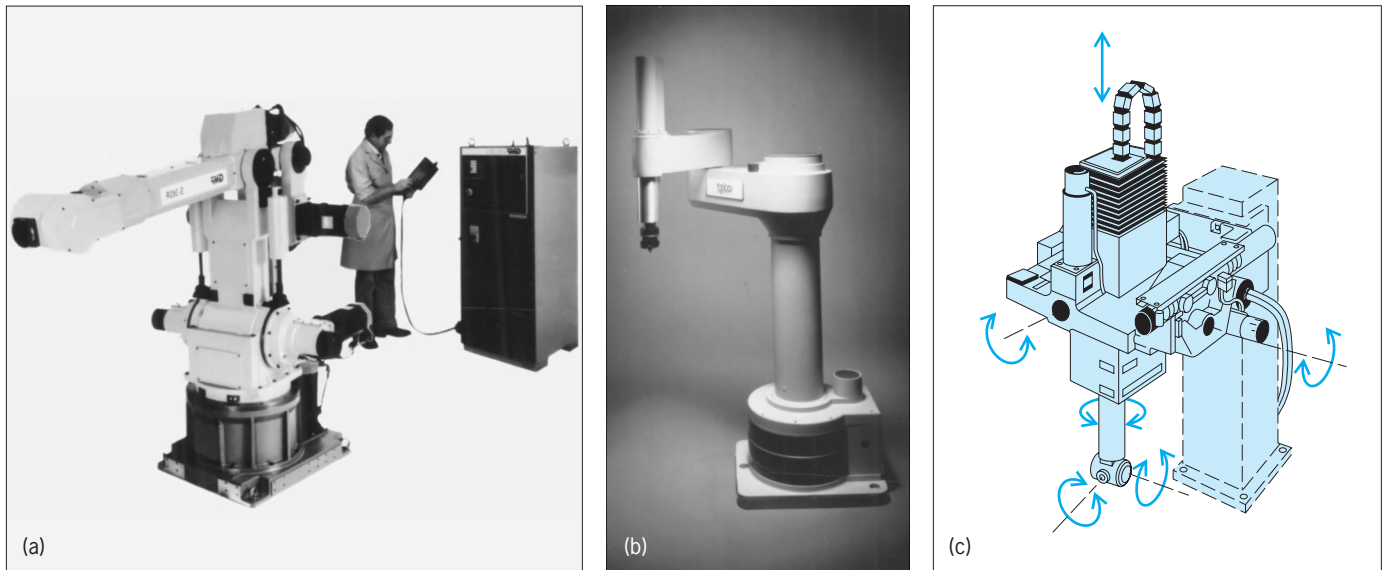
Fig. 1. Industrial robots. (a) Articulated, with rotary joints (GM Fanuc Robotics Corp.). (b) Selective compliance assembly robot arm (SCARA) configuration (Adept Technology, Inc.) (c) Overhead gantry.
