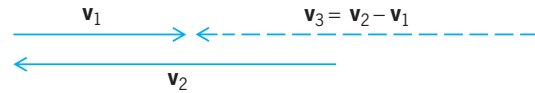
Fig. 3. Relative velocity of two bodies moving in opposite directions; that is, velocities are antiparallel.
