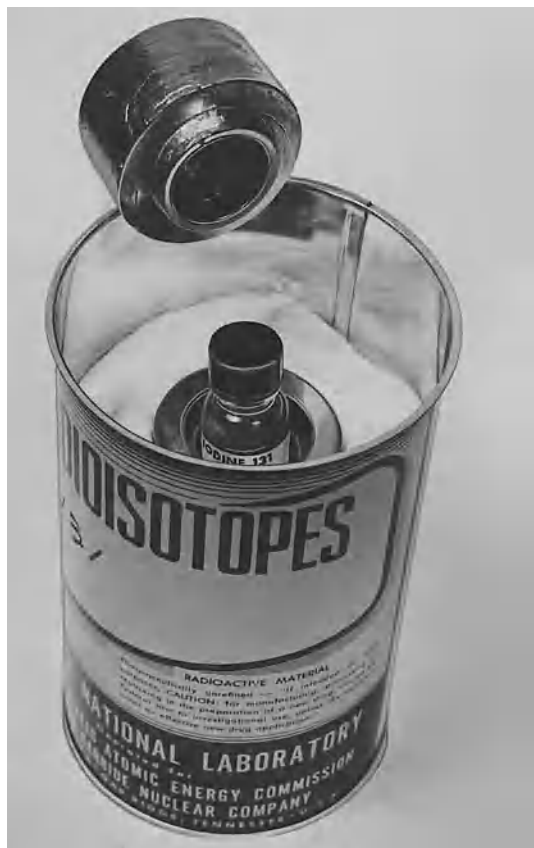
Fig. 3. Nonreturnable shipping container for radioisotopes. (Oak Ridge National Laboratory)
