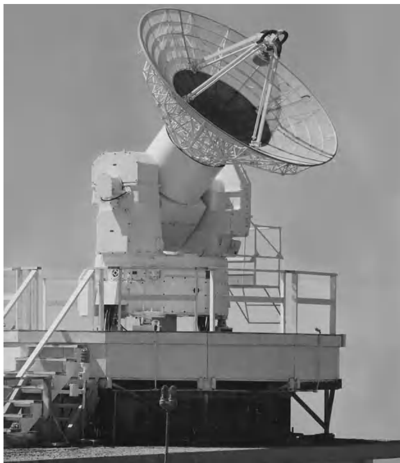
Fig. 5. AN/FPS-16 tracking radar, a very accurate monopulse radar, operating in the C-band, installed at more than 50 sites around the world. (RCA Corp.)
